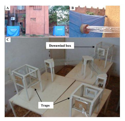
**Figure 1. The bioassay.** (A) The two tents set up outdoors and connected to the two traps of the Y-olfactometer by lay-flat tubing, and the olfactometer room located between the two tents. (B) Fan drawing air from a tent to the olfactometer via lay-flat tubing. (C) The Y tube-olfactometer. doi:10.1371/journal.pone.0009546.g001
