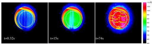
Fig. 3. Temperature field in Kelvin and studied area (white circle) for one test at 55 kW/m<sup>2</sup>.
