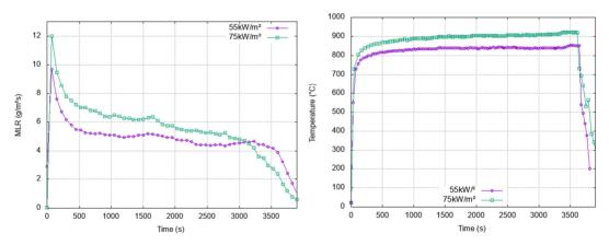
Fig. 5. MLR and surface temperature for tests with sample ignition.
