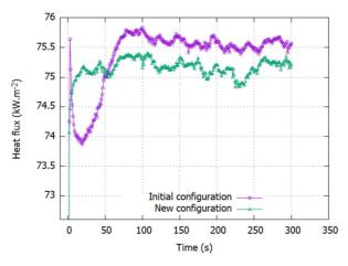
Fig. 2. Heat flux measured for the initial and new configurations (75 kW/m<sup>2</sup>).
