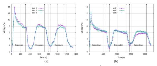
Fig. 8. MLR of tests with an exposure of 75 kW/m<sup>2</sup> (a) 5 min; (b) 10 min.
