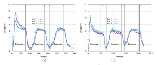
Fig. 7. MLR of tests with an exposure of 55 kW/m<sup>2</sup> (a) 5 min; (b) 10 min.
