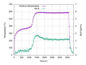
Fig. 4. MLR and surface temperature for tests without ignition
