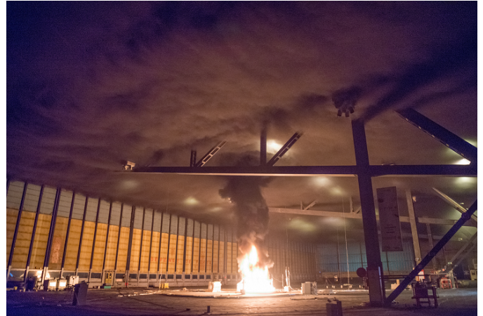
Figure 1: View of a 6\text{ m}^2 kerosene pool fire in Orly. The opacimetry setup (behind brick walls) can be seen to the left and right of the fire.
