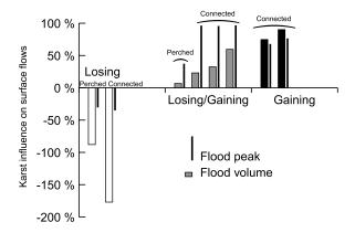
**Figure 6.** Karst influence on the flash flood peak and the cumulative runoff at the exit of the karst aquifer for various types of hydrodynamic connections and interactions between SW and GW using the 8 flood events recorded in the Coulazou River. See text for discussion for relevance of a losing or gaining stream for these computed karst influences on surface flows.
