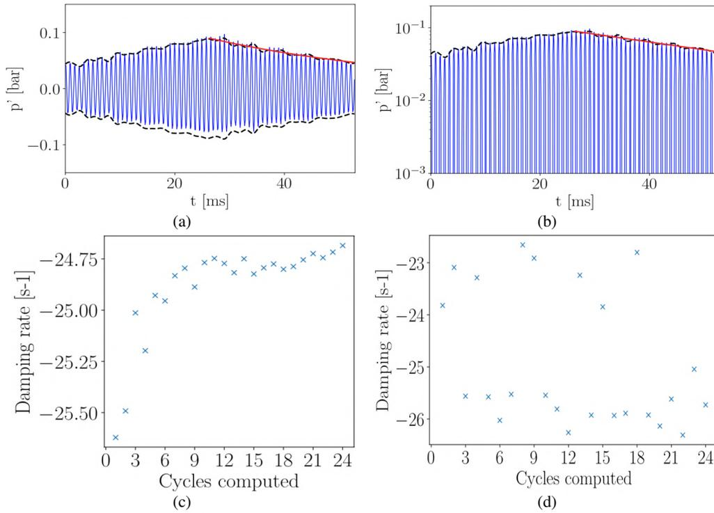
Figure 10: Damping rate determination for the 1T simulated mode, using the pressure signal from HFc1 probe. (a) Average cycle of the pressure signal (—), envelope (---), exponential fit (—) (b) Logarithm of the average cycle (—) (c) Damping rate determined by the average cycle method with respect to the number of cycles computed (d) Damping rate evaluated for each cycle and used by the statistical method with respect to the number of cycles computed
