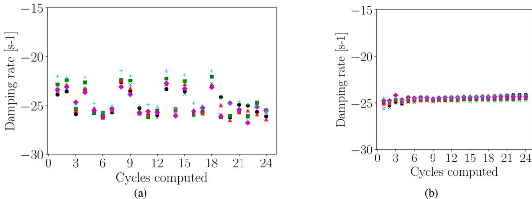
Figure 12: Dispersion with probe location of the damping rate using a) the statistical method and b) the average-cycle method.  $\times$  HFc1,  $\bullet$  HFc2,  $\square$  HFc3,  $\triangle$  HFc4,  $\diamond$  HFc5,  $+$  HFc6
