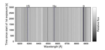
**Figure 7.**  $600 \times 5$  s SALT RSS red spectra, covering 6137–6953 Å, of TYC 8332-2529-1 taken on 2019 March 1. The absorption lines include the narrow H $\alpha$  line (right of centre), the telluric oxygen *B* band (far right, marked with  $\bigoplus$ ) and many other photospheric lines. Each spectrum was normalized to account for slit losses.
