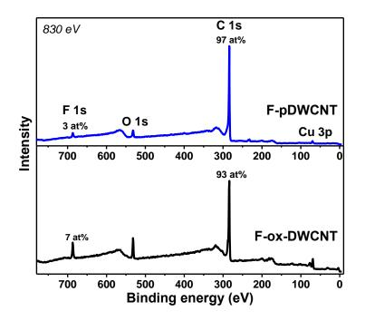
Fig. S1. XPS overall spectra of F-pDWCNTs and F-ox-DWCNTs
