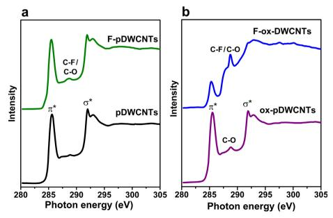
Fig. 4. NEXAFS C K-edge spectra of pDWCNTs (a) and ox-DWCNTs (b) before and after fluorination (F-pDWCNTs and F-ox-DWCNTs).
