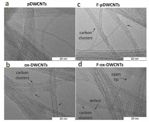
Fig. 1. TEM images of air-purified DWCNTs (a, pDWCNTs), oxidized/purified DWCNTs (b, ox-DWCNTs), fluorinated pDWCNTs (c, F-pDWCNTs) and fluorinated ox-DWCNTs (d, F-ox-DWCNTs).
