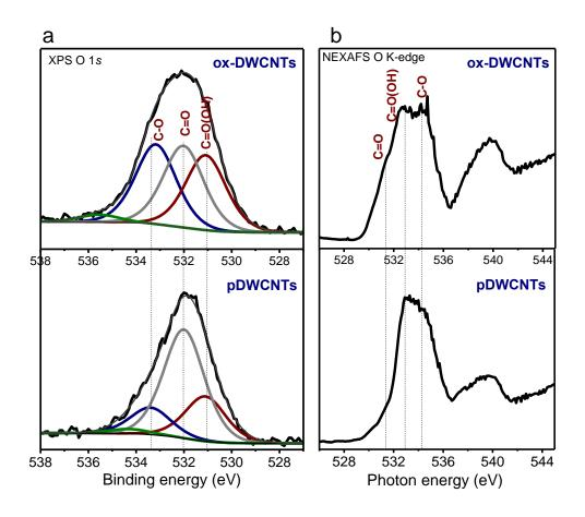
Fig. S2. XPS O1s spectra (a) and NEXAFS OK-edge spectra (b) of pDWCNTs and ox-DWCNTs
