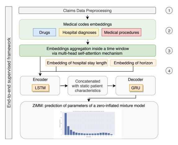
Figure 1: Architecture of the ZiMM Encoder-Decoder end-to-end architecture. A detailed graphical representation of Steps 2-4 is shown in Figure 3 below.
