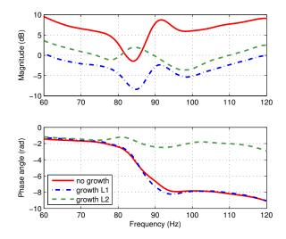
Figure 3: (Color online) Example of measured frequency response functions (FRF) of the vocal fold replica, in healthy and pathological configurations, at the water pressure  $P_w = 25 \text{ cm H}_2\text{O}$ .
