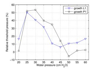
Figure 7: (Color online) Oscillation threshold pressure with the lead (L1) and plasticine (P1) growths, relative to their respective reference series without growth (Fig. 6). The series with growth L1 is the same as in Fig. 5 in the high frequency regime.
