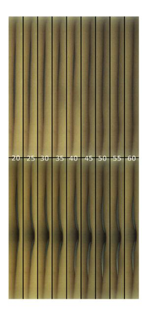
Figure 8: (Color online) Photographs of the glottis without growth (first row) and with growth L1 (second row) for water pressure inside the latex tubes  $P_w$  varying from 20 to 60 cm H<sub>2</sub>O. These photographs are flipped (90°): the vocal fold on the left side of each photograph was the upper vocal fold during the experiment.
