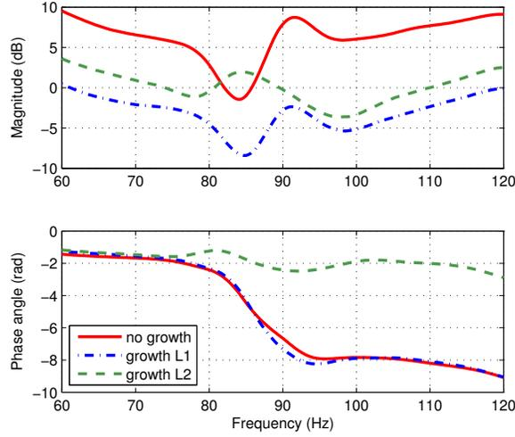
Figure 3: (Color online) Example of measured frequency response functions (FRF) of the vocal fold replica, in healthy and pathological configurations, at the water pressure  $P_w = 25$  cm H<sub>2</sub>O.
