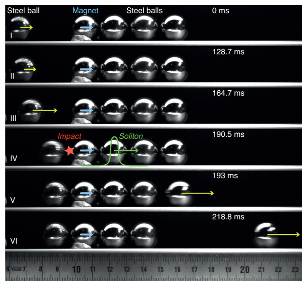
FIG. 1. Time sequence (from top to bottom) showing acceleration in the magnetic cannon. A line of three steel balls initially stuck to the right of a strong permanent magnet, loosely fixed on a rail, is impacted by a steel ball coming from the left hand side and accelerated in the magnetic field of the magnet. Momentum is transferred into the chain and the last ball on the right is ejected at high velocity. Images from a 2048x360 pixel film acquired at 400 frames per second.
