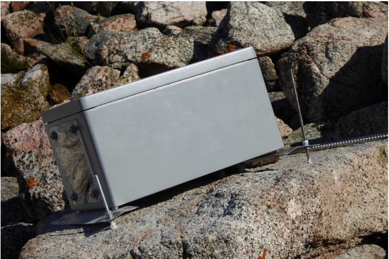
Figure 12. The box is bolted to a boulder.
