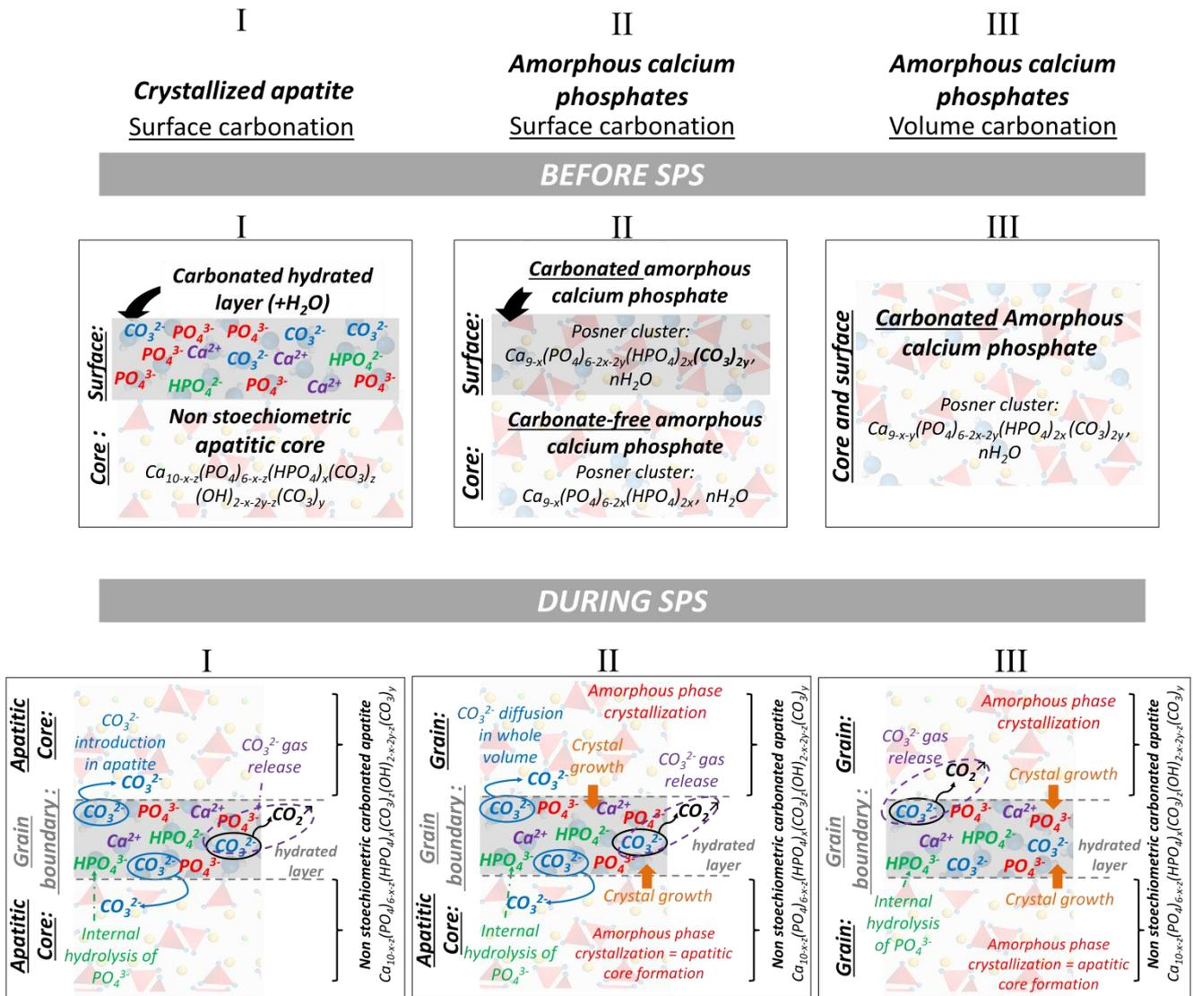
Figure 10: Schematic representation of different states of carbonated calcium phosphates before and during SPS.
