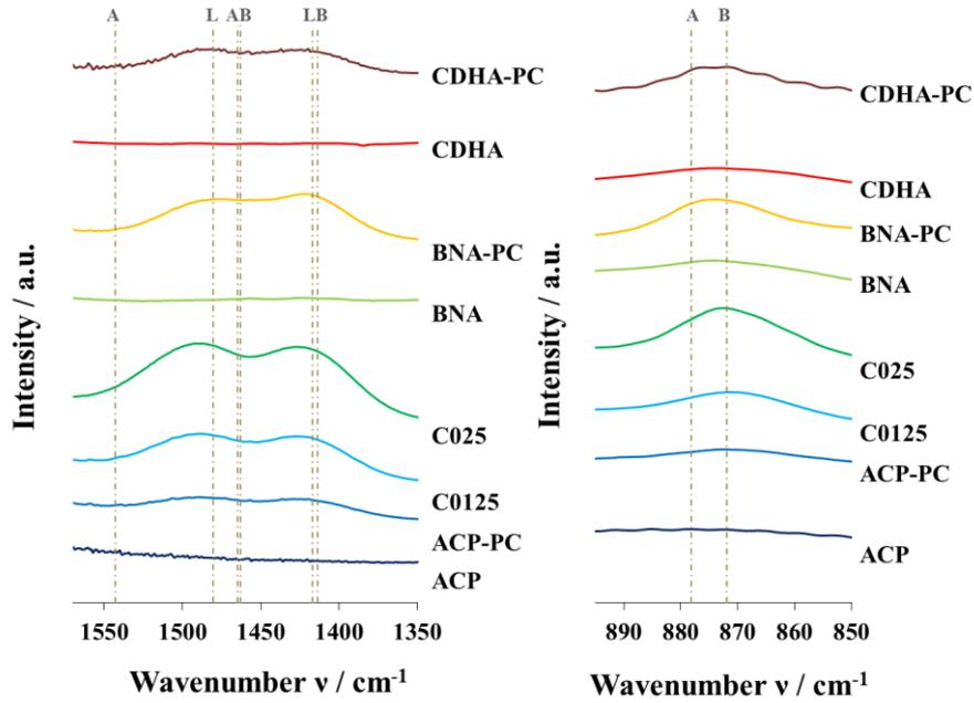
Figure 2: FTIR zooms on  $\nu_3$  (1570-1350  $\text{cm}^{-1}$ ) and  $\nu_2$  (895-850  $\text{cm}^{-1}$ )  $\text{CO}_3$  bands of powders (Contributions are denoted A for A-site, B for B-site and L for labile carbonate).
