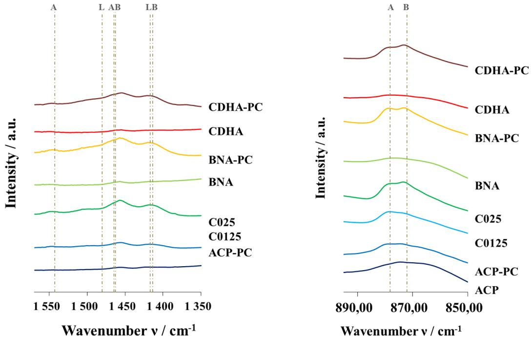
Figure 6: FTIR zooms on  $\nu_3$  (1570-1350  $\text{cm}^{-1}$ ) and  $\nu_2$  (895-850  $\text{cm}^{-1}$ ) bands of SPS ceramics (Contributions are denoted A for A-site, B for B-site and L for labile carbonate).
