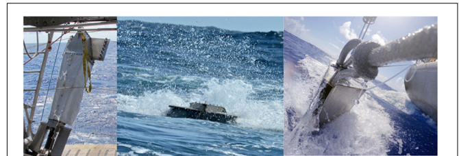
FIGURE 4 | Surface net and water samplers. The High Speed Net on board and in work ( left and middle ), and the “Dolphin” ( right ) deployed simultaneously. The Dolphin is connected to a large volume peristaltic pump installed on the deck for surface water sampling (Photos from left to right F. Lombard, F. Aurat, J.M. Flores.)
