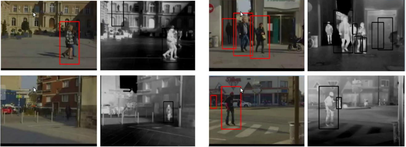
Fig. 5. Examples of detections obtained on visible images and far-infrared images. We can see that the strengths and weaknesses of the far-infrared and the visible detectors are different.
