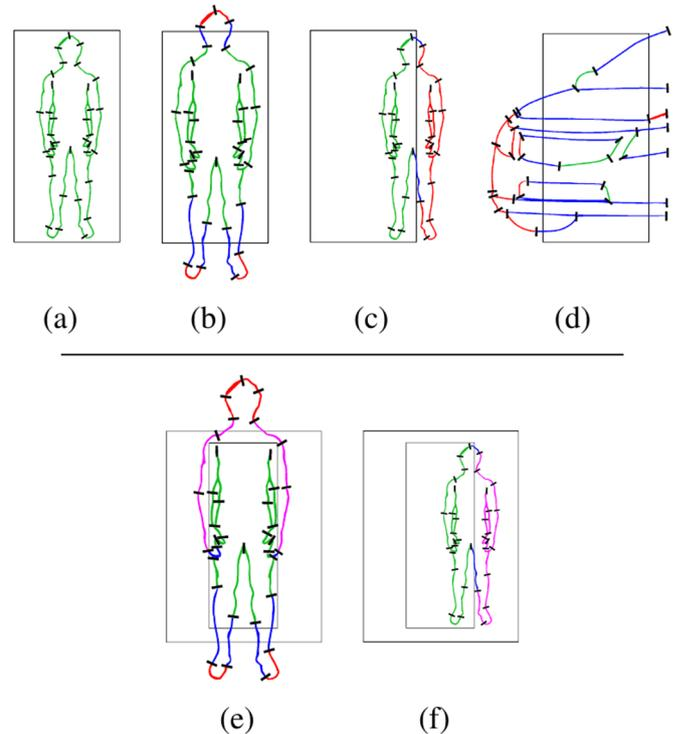
**Fig. 6.** Above: contours used for the EB score. In green: internal contours, in blue: intersecting contours and in red: external contours. From (a) to (d): the EB score decreases (the number of internal contours decreases and the number of traversing contours increases). Below: the additional contours used for the CAO score. In pink: affiliated external contours. In (e) and (f): as the number of affiliated external contours increases the CAO score decreases.
