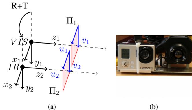
**Fig. 1.** (a) The layout of our stereo acquisition system. VIS and IR are respectively the visible and the infrared camera,  $\Pi_1$  and  $\Pi_2$  are the image planes of respectively camera VIS and IR.  $R$ : rotation matrix from camera VIS to camera IR,  $T$ : translation matrix from camera VIS to camera IR. (b) Picture of our stereoscopic system.
