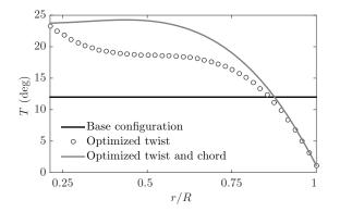
Figure 5: Twist distribution laws of the successive rotors.
