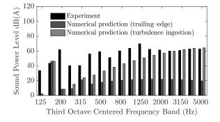
Figure 16: Sound power level of the acoustic spectrum of the final optimized rotor for a 2 N thrust.
