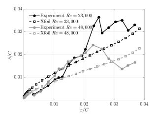
Figure 3: Boundary Layer thickness on a NACA 0012 at Reynolds numbers Re = 23,000 and Re = 48,000 and a 6° angle of attack between Xfoil prediction and experiments by Kim *et al.* [12].
