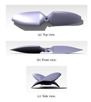
Figure 17: CAD representation of the optimized rotor. It radiates 10 dB(A) less and consummes 4 W less for the same thrust production.
