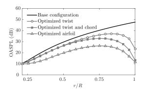
Figure 11: Spanwise blade element contribution to the overall sound pressure level (OASPL) for a 2 N thrust for the successive rotors. Numerical prediction from the trailing–edge noise model.
