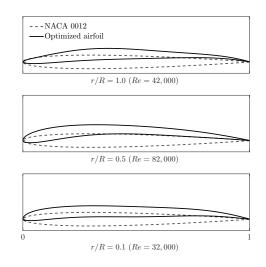
Figure 8: Optimized airfoil sections for the fourth rotor compared with the base configuration (NACA 0012).
