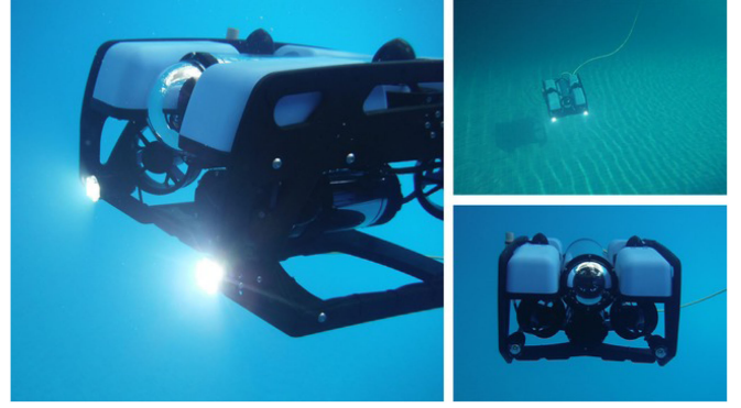
Fig. 4. Underwater vehicle BlueROV2 during a mission. The BlueROV2 was modified in this work to accomplish fully autonomous operation as an AUV instead of remotely operation as a ROV.
