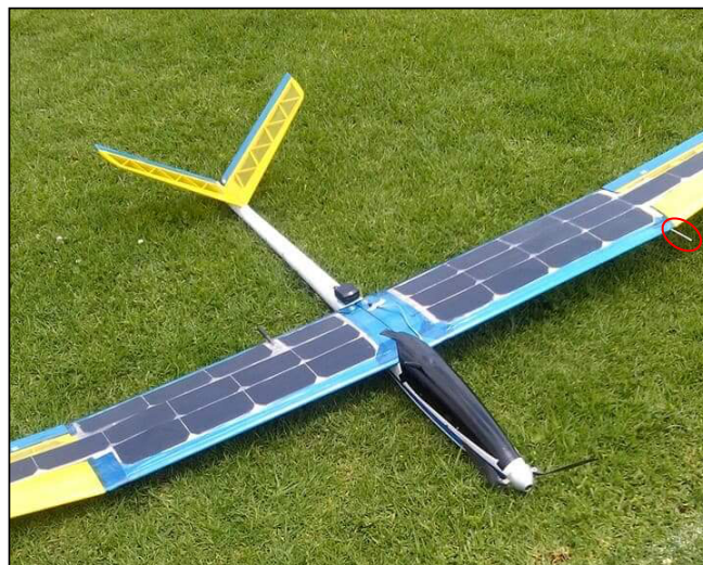
Figure 12. SUAV in the flight field, doing a pre-flight check. Pitot-tube is marked in red.
