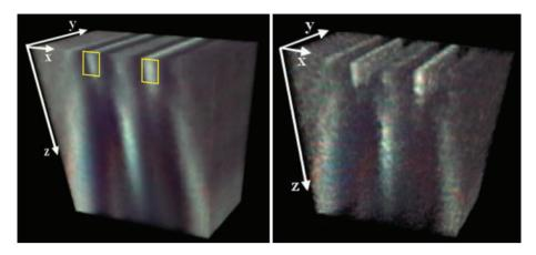
**Figure 6:** White-light 3D intensity distributions diffracted by a pair of parallel polymer lines separated by 2  $\mu$ m. Left: raw z-stack images. Right: deconvoluted z-stack images. Yellow rectangles represent line profiles (W=0.4  $\mu$ m and H=0.9  $\mu$ m).
