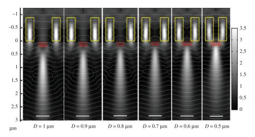
**Figure 4:** Diffraction intensity patterns generated by pairs of dielectric rectangles (W = 0.3  $\mu$ m, H = 0.9  $\mu$ m, n =1.52) for separating distances D = 1  $\mu$ m, 0.9  $\mu$ m, 0.8  $\mu$ m, 0.7  $\mu$ m, 0.6  $\mu$ m, 0.5 $\lambda$ .
