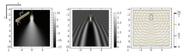
**Figure 1:** Calculated intensity patterns and phase map generated by a dielectric rectangular structure ( $W = \lambda$ ,  $H = 2\lambda$ , n = 1.4) in air with an incident plane wave (in-plane polarization).
