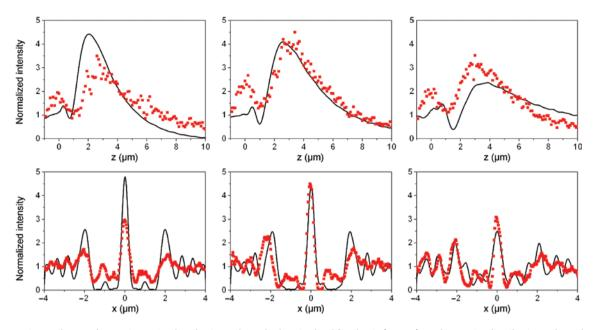
**Figure 8:** First and second rows: intensity distributions along the longitudinal focal axis (x = 0, z), and intensity distributions along the lateral focal axis ( $x, z = Z_z$ ).
