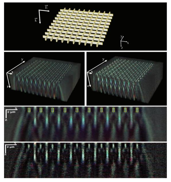
**Figure 9:** First row: The schematic of the polymer grid. Second row: white-light 3D intensity distributions diffracted by a grid of parallel polymer lines separated by 2 µm into a borosilicate substrate.
