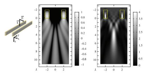
**Figure 2:** Calculated intensity patterns generated by a pair of dielectric rectangular structures ( $W = \lambda$ ,  $H = 2\lambda$ , spacing  $D = 4\lambda$ , n = 1.4 in air with an incident plane wave (in-plane polarization).
