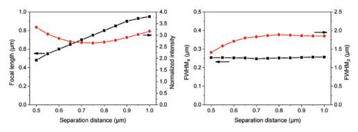
**Figure 5:** Evolution of optical characteristics with respect to the decrease of the separation distance below 1 µm. Left: variations of focal lengths (black squares) and normalized maximum intensities (red circles) with the separation distance. Right: lateral resolution FWHM<sub>x</sub> (black squares) and depth of focus FWHM<sub>z</sub> (red circles) variations with the separating distance.
