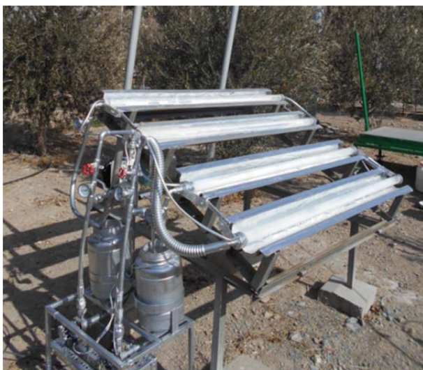
Figure 1: The Solar reactor CPC unit of 4 borosilicate glass tubes equipped with tanks and pumps for recirculation of AMX solutions.
