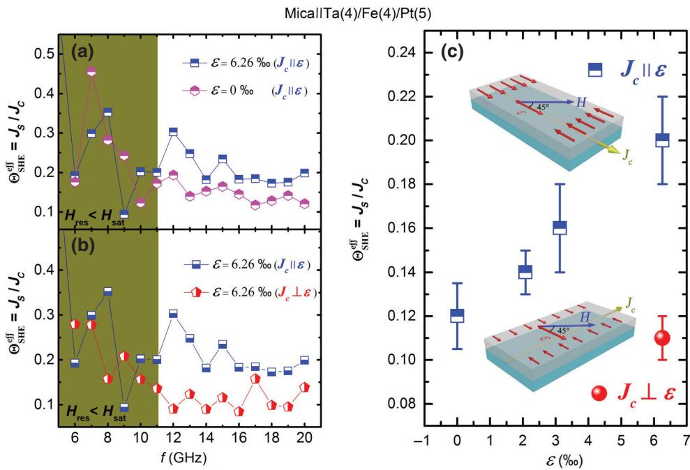
FIG. 4. (a),(b) Determination of the effective spin Hall angle according to Eq. (3), which is reliable only when  $H_{\text{res}} > H_{\text{sat}}$  [32]. (c) Strain dependence of the effective spin Hall angle.
