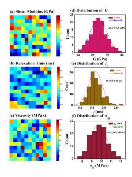
**Fig. 36.** Mapping of (a) local shear modulus, (b) local relaxation time and (c) local viscosity of the Zr-based amorphous alloy at the indentation load of 800 mN andthe scanning space of 100 nm. On the right are the corresponding statistical distribution of (d) local shear modulus, (e) local relaxation time and (f) local viscosity. The dashed lines are the Gaussian fitting to the experimental data [245]. Reprinted from reference [245], copyright (2014), with permission from Elsevier.
