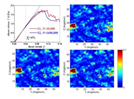
**Fig. 50.** (a) Shear stress-strain curves of  $Cu_{50}Zr_{50}$  amorphous alloy for S1 and S2 at 1 K with strain rate  $1.0 \times 10^8 \text{ s}^{-1}$  [210]. The yielding strain is about4%. (b)–(d) Contour maps of the same slice (5 °A, ~2*d*Cu) from three independent shear runs to the yielding point (4%) in S1. The color scale represents the atomic non-affine displacement. Reprinted figures with permission from reference [210], copyright (2016) by the American Physical Society.
