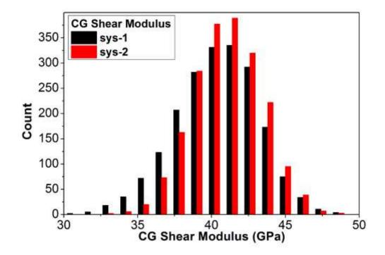
**Fig. 48.** The distribution of the first nearest neighbor coarse-grained (CG) shear modulus, in both systems [269]. Black bars are for system I, and red bars represent system II. Reprinted figures with permission from reference [269], copyright (2014) by the American Physical Society.
