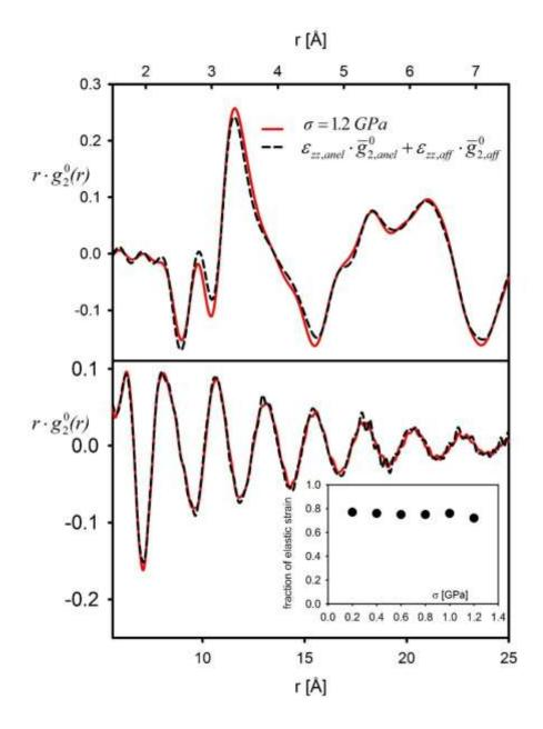
**Fig. 31.** The l=2 component of the PDF,  $g_2^0(r)$ , at1.2 GPa, fitted to the combined PDF for affine and creep(anelastic) deformation, Eq. (4). The inset shows the fraction of elastic strain compared to the total apparent strain. It appears constant of applied external stress up to 1 GPa, and on average it is about 76%. The rest, 24%, is the
