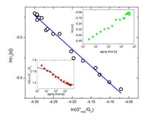
**Fig. 21.**  $\ln(\tau_{\beta})$  vs  $\ln(G''_{max}/G_U)$  for La<sub>60</sub>Ni<sub>15</sub>Al<sub>25</sub> amorphous alloy aged at 433K with different aging times (the testing temperature is 343K) [184]. Reprinted from [184], with the permission of AIP Publishing.
