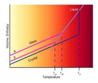
**Fig. 1.** Sketch of glass formation. Volume and enthalpy decrease as the liquid is cooled. For a high cooling rate glass transition takes place at a higher temperature –  $T_{ga}$  – than for a lower quenching rate –  $T_{gb}$  –. Reprinted by permission from Nature, reference [83], copyright (2001).
