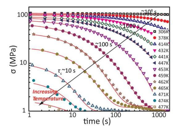
Fig. 3. Evolution of stress relaxation as function of temperature of  $La_{60}Ni_{15}Al_{25}$  metallic glass, taken from reference [95]. Reprinted by permission from Nature
