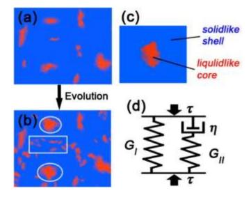
**Fig. 67.** (a) Schematic illustration of the zones of local heterogeneity being activated under stress in metallic glasses (the red regions represent the liquid-like cores and the blue surroundings the elastic matrix); (b) illustration of the evolution of the structural heterogeneity; (c) sketch of the core–shell deformation unit in metallic glasses; and (d) the three-parameter viscoelastic model[218]. Reprinted from reference [218], copyright (2013), with permission from Elsevier.
