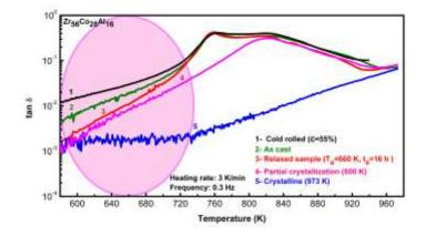
**Fig.15.** Evolution of the internal friction with the temperature in  $Zr_{56}Co_{28}Al_{16}$  amorphous alloy at different states [134]: (1) 55% thickness reduction after cold-rolling, (2) as-cast sample (3) after structural relaxation (annealing temperature is 660 K with annealing for 16 hours), (4) formation of partial crystallization (heating to 800 K with a heating rate of 3 K/min). Reprinted from reference [134], copyright (2014), with permission from Elsevier.
