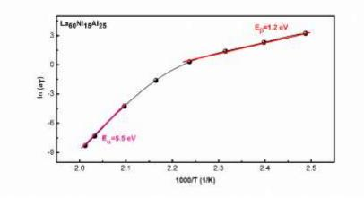
**Fig. 11.** Shift factor obtained by TTS principle for  $La_{60}Ni_{15}Al_{25}$  amorphous alloy. Reprinted from reference [94], with the permission of AIP Publishing.
