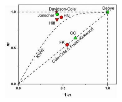
**Fig. 9.** Parameters of relaxation functions fitted to the mechanical relaxation data of  $Zr_{40}Ti_{25}Cu_8Be_{27}$  metallic glass. *m* and 1-*n* correspond to the low and high-frequency slopes of the log-log plot of the loss modulus. From ref. [116]. Reprinted from reference [116]. Copyright (2017), with permission from Elsevier.
