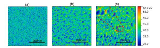
**Fig. 42.** Energy dissipation images of  $Zr_{70}Ni_{30}$  TFMG and the corresponding 2D FFT patterns [264]. (a-c) Are energy dissipation images obtained at the as-deposited state, at the indentation area with the load of 40 mN and 3 N, respectively. The zoom-in image of the area boxed in red in (c) clearly shows the quadrupolar characteristics of HDR. Reprinted by permission from Macmillan Publishers Ltd: Scientific Reports, reference[264], copyright (2016).
