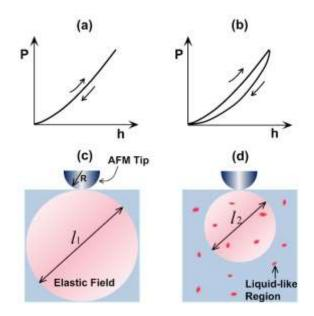
**Fig. 38.** The schematic illustrations of the mechanical response for elastic and viscoelastic material under AFM tip tapping [264]. Reprinted by permission from Macmillan Publishers Ltd: Scientific Reports, reference[264], copyright (2016). The typical load-displacement (*P-h*) curve for (a) elastic and (b) viscoelastic material; (c) the elastic interaction volume within an elastic material with its size  $l_1$  correlated with
