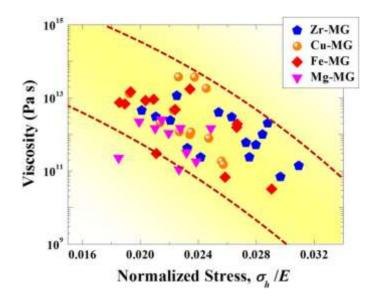
**Fig.75.** The extracted viscosity of the steady-state viscous flow showing a "shear thinning" behavior of the different types of amorphous alloys prior to shear instability[446]. Reprinted from reference[446], with the permission of AIP Publishing.
