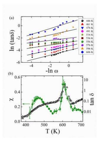
**Fig. 66.** (a) Variation of  $\ln(\tan \delta) vs \ln \omega$  at different temperatures of  $Pd_{43}Ni_{10}Cu_{27}P_{20}$  amorphous alloy; (b) Temperature dependence of the correlation factor  $\chi$  and the loss factor tan  $\delta$ . Adapted with permission from reference [382]. Reprinted from reference [382], with the permission of AIP Publishing.
