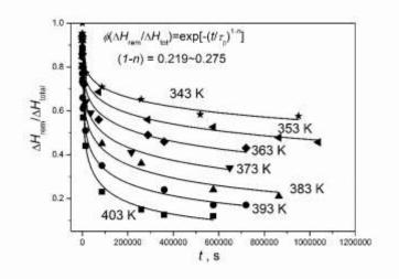
Fig. 25. Dependence of normalized remaining enthalpy on annealing time at temperatures below  $T_g$  for La<sub>55</sub>Al<sub>25</sub>Ni<sub>20</sub> metallic glass. Reprinted with permission from reference [197]. Copyright (2016) American Chemical Society.
