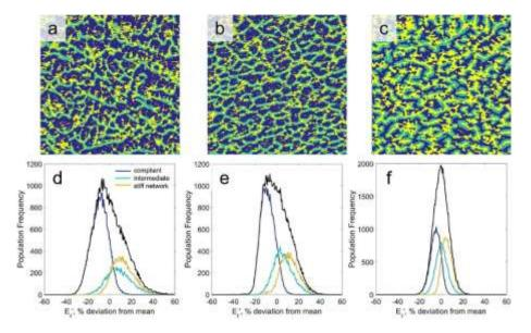
**Fig.78.** K-means clustering analysis for characterization of elastic microstructure[449]. (a-c) Example tricolor representations of the modulus maps with the pixels grouped according to the modulus category (blue = compliant, green = intermediate, and
