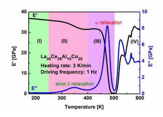
Fig. 17. The temperature dependence of the storage modulus E' and loss modulus E'' with temperature in La<sub>30</sub>Ce<sub>30</sub>Al<sub>15</sub>Co<sub>25</sub> amorphous alloy. Reprinted from reference[150], copyright (2019), with permission from Elsevier.
