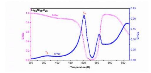
**Fig. 4.** Storage modulus and loss modulus of a  $La_{60}Ni_{15}Al_{25}$  metallic glass as a function of temperature. Reprinted from[94], with the permission of AIP Publishing.
