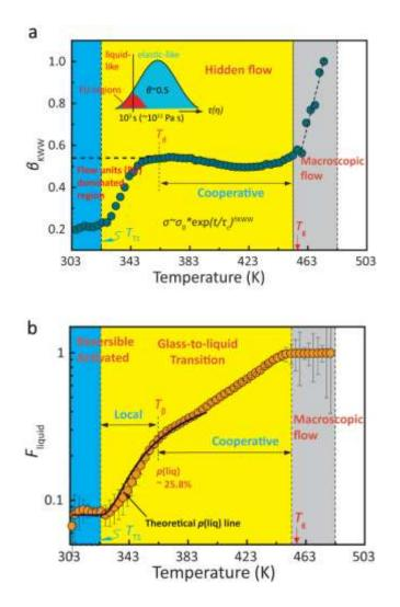
Fig. 57. (a) Evolution of  $\beta_{KWW}$  values (dark green circles) of La<sub>60</sub>Ni<sub>15</sub>Al<sub>25</sub> metallic glass based on fitting from stress relaxation experiments at different temperatures [95].
