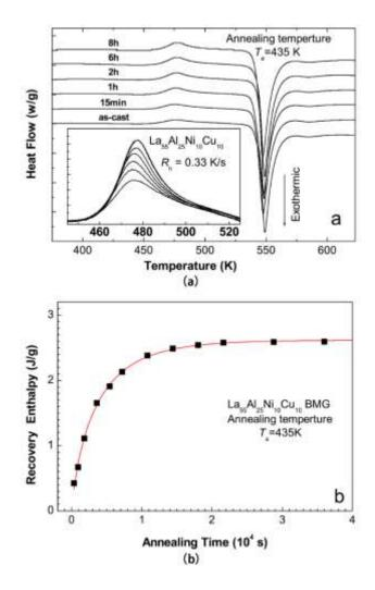
**Fig. 24.** (a) DSC curves of  $La_{55}Al_{25}Ni_{10}Cu_{10}$  amorphous alloy for different annealing times. (b) Recovery enthalpy obtained from the DSC experimental data. Reprinted by permission from [195], Springer, copyright (2008).
