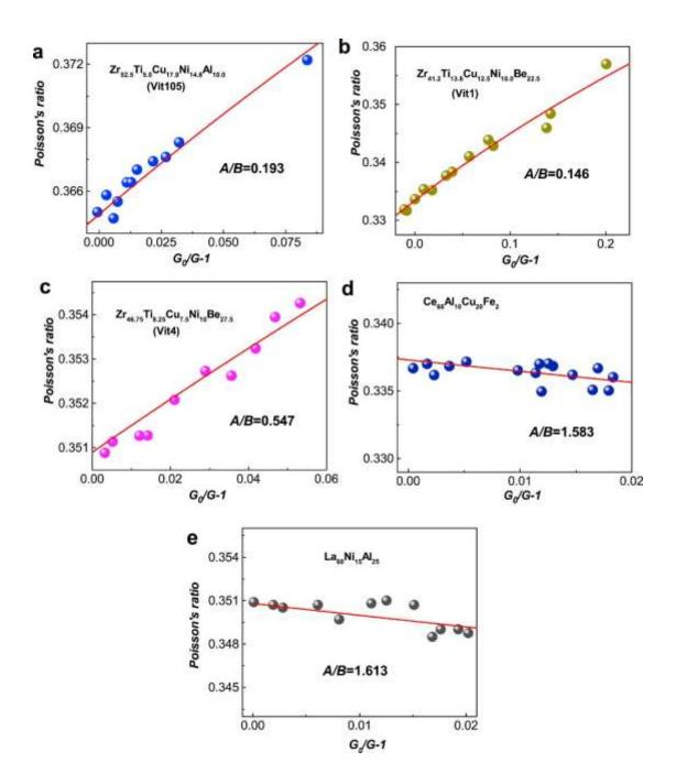
**Fig. 68.** The plot of measured Poisson's ratio, v, versus ( $G_0/G-1$ ) upon annealing for different amorphous alloys: (a) Vit105; (b) Vit1; (c) Vit4; (d) Ce<sub>68</sub> Al<sub>10</sub>Cu<sub>20</sub> Fe<sub>2</sub>; (e) La<sub>60</sub>Ni<sub>15</sub>Al<sub>25</sub>. All data were well fitted by equation (5-2), with the fitting values A/B listed [406]. Reprinted from reference [406], copyright (2016), with permission from Elsevier.
