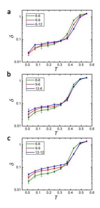
**Fig. 51.** The internal friction measured by MD-DMA [256]. (a)-(c) The internal frictions for models with different attractive interactions, repulsive interactions and both attractive and repulsive interactions, respectively. Low-temperature relaxation dynamics is enhanced with the increase of interaction stiffness. Published with permission of Royal Society of Chemistry, from reference [256], copyright (2016). Permission conveyed through Copyright Clearance Center, Inc.
