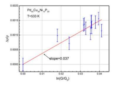
Fig. 62. Relative density change upon structural relaxation of the  $Pd_{40}Cu_{30}Ni_{10}P_{20}$
