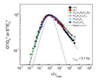
Fig. 7. Normalized loss modulus peak of amorphous alloys at a temperature were the peak maximum is near 0.1 Hz. Experimental data is compared to Debye and HN functions, the latter with parameters  $\alpha = 0.95$  and  $\gamma = 0.41$ . Reprinted from reference [111], with the permission of AIP Publishing.
