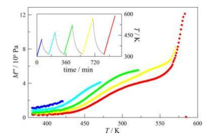
**Fig. 18.** Loss modulus of  $Pd_{42.5}Ni_{7.5}Cu_{30}P_{20}$  measured at a constant frequency of 1 Hz during consecutive heating runs. The applied thermal protocol is shown in the inset. Reprinted with permission from reference [165]. Copyright (2016) American Chemical Society.
