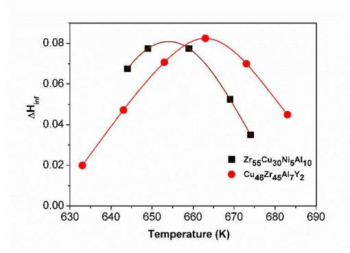
**Fig. 26.** Enthalpy relaxation in  $Zr_{55}Cu_{30}Al_{10}Ni_5$  and  $Cu_{46}Zr_{45}Al_7Y_2$  amorphous alloys after annealing at different temperatures [199]. Reprinted from reference [199], copyright (2011), with permission from Elsevier.
