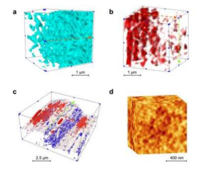
**Fig. 32.** Hierarchical microstructure of as-quenched metallic glasses [29]. (a) The low-density regions in  $Pd_{40}Ni_{10}Cu_{30}P_{20}$  metallic glass. (b) The high-density regions in  $Zr_{52.5}Ti_5Cu_{17.9}Ni_{14.6}Al_{10}$  metallic glass. (c),The high-density regions (marked by red color) and low-density regions (marked by blue color) in  $Zr_{64.13}Cu_{15.75}Ni_{10.12}Al_{10}$  metallic glass. (d) The 3D fine structure reconstructed by nano-CT for
