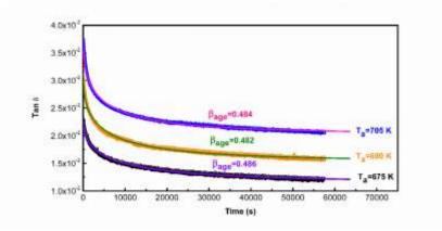
Fig. 27. Time dependence of the loss factor tan  $\delta$  in Zr<sub>56</sub>Co<sub>28</sub>Al<sub>16</sub> amorphous alloy during structural relaxation at various temperatures [134]. Reprinted from ref. [134], Copyright (2014), with permission from Elsevier.
