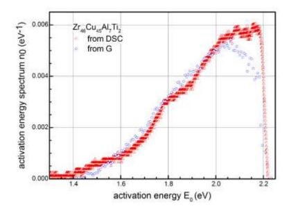
**Fig. 59.** Activation energy spectra of structural relaxation reconstructed from independent shear modulus and calorimetry data [368]. Reprinted from reference [368], copyright (2016), with permission from Elsevier.
