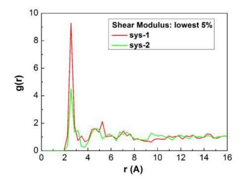
**Fig. 46.** The PDF of a subset group of atoms with lowest 5% shear modulus in two systems [269]. Red curves are for system I, green curves are for system II. Reprinted figures with permission from reference [269], copyright (2014) by the American Physical Society.
