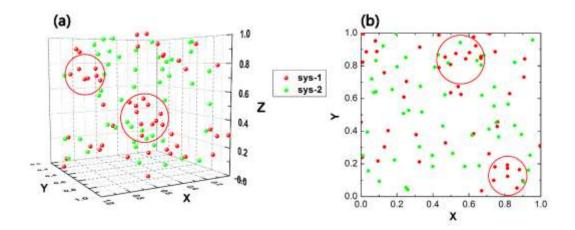
Fig. 47. The positions of the atoms with the lowest 2.5% shear modulus [269], in 3D display (a), and 2D projection in X-Y plane (b). Atoms in red are for system I, and atoms in green are for system II. Reprinted figures with permission from reference [269], copyright (2014) by the American Physical Society.
