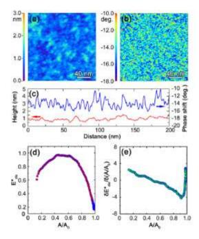
Fig. 39. (a) The height image with rms roughness of ~0.3 nm, (b) the phase shift
