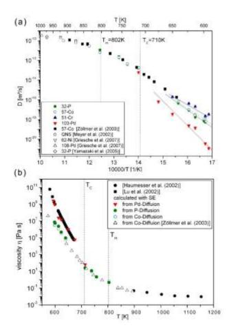
**Fig. 28.** (a) Arrhenius plot for diffusion of Pd, P, Co and Cr in liquid  $Pd_{43}Cu_{27}Ni_{10}P_{20}$  alloys.  $T_m$  and  $T_c$  are the melting and critical temperature of the mode coupling theory, respectively. (b) Diffusion-viscosities of Pd, Co, and P computed from the Stokes-Einstein relation compared to the liquid viscosity. Reprinted figures with permission from reference [206], copyright (2010) by the American Physical Society.
