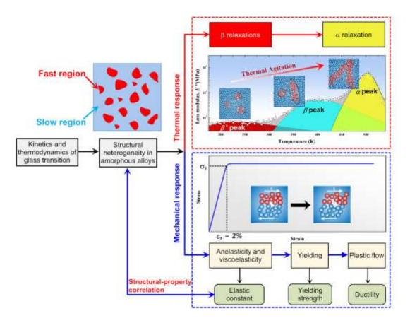
**Fig. 1.** The correlation between mechanical relaxations and mechanical properties of amorphous alloys. The mechanical spectrum adapted from reference[61]. Reprinted by permission from Macmillan Publishers Ltd: Nature Communications, reference[61], copyright (2015).
