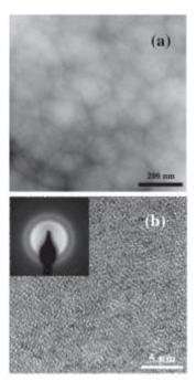
**Fig.77.** (a) A scanning transmission electron microscope (TEM) image of the as-cast  $La_{68.5}Ni_{16}Al_{14}Co_{1.5}$  amorphous alloy. (b) A high-resolution TEM micrograph of the as-cast  $La_{68.5}Ni_{16}Al_{14}Co_{1.5}$  amorphous alloy; the inset shows the selected-area electron diffraction. Reprinted figures with permission from reference [448], copyright (2012) by the American Physical Society.
