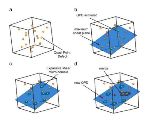
**Fig. 63.** Schemes corresponding to the quasi-point defect model (a) Quasi-point defects in amorphous materials(b), (c) and (d) activation of these QPD and growth of sheared micro-domains (SMD) induced by application of a stress [379]. Reprinted from ref. [379], copyright (2011), with permission from Elsevier.
