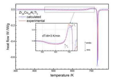
**Fig. 60.** Experimental DSC traces for  $Zr_{46}Cu_{45}Al_7Ti_2$  amorphous alloys and the heat flow calculated with Eq. (4-5) [370]. Reprinted by permission from Macmillan Publishers Ltd: Scientific Reports, reference[370], copyright (2016).
