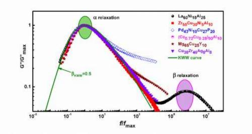
**Fig. 8.** Normalized loss modulus peak of amorphous alloys at a temperature were the peak maximum is near 0.1 Hz. Experimental data is compared to the transform of a KWW function with  $\beta_{KWW} = 0.5$  [112]. Reprinted from reference [112], copyright (2014), with permission from Elsevier.
