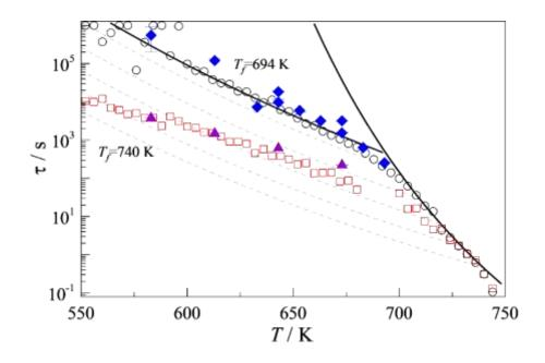
**Fig. 12.** Relaxation times obtained by dynamic (open circles) and quasi-static (full symbols) mechanical relaxation of as-quenched (red and purple symbols) and annealed (black and blue symbols)  $Cu_{46}Zr_{46}Al_8$  metallic glass. Reprinted From ref. [115] Copyright (2015), with permission from Elsevier.
