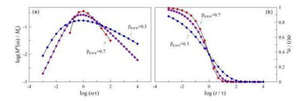
**Fig. 6.** Left: Relaxation peaks obtained by equation 2-4 from KWW correlation functions. The values of stretching exponent are  $\beta_{KWW} = 0.3$  (blue),  $\beta_{KWW} = 0.5$  (purple) and  $\beta_{KWW} = 0.7$  (red). Right: Corresponding KWW correlation functions.
