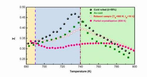
**Fig. 65.** Evolution of the correlation factor  $\chi$  with temperature in Zr<sub>56</sub>Co<sub>28</sub>Al<sub>16</sub> bulk metallic glass at different states [134]. Reprinted from reference [134], copyright (2014), with permission from Elsevier.
