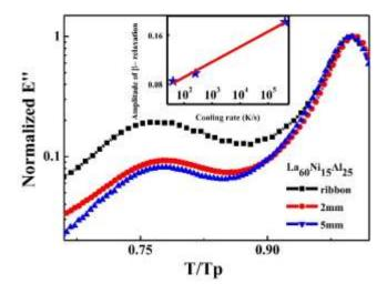
**Fig. 22.** The normalized loss modulus of the La<sub>60</sub>Ni<sub>15</sub>Al<sub>25</sub> metallic glass for the ribbon and rod ( $T_p$  is the peak maximum of the slow  $\beta$  relaxation). The inset is the quenching rate dependent amplitudes of the slow  $\beta$  relaxation [188]. Reprinted from reference [188], copyright (2014), with permission from Elsevier.
