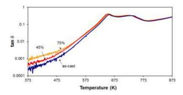
**Fig. 14.** Effect of the cold-rolling ratio ( $\varepsilon = 45\%$  and  $\varepsilon = 75\%$ ) on loss factor tan  $\delta$  of Ti<sub>40</sub>Zr<sub>25</sub>Ni<sub>8</sub>Cu<sub>9</sub>Be<sub>18</sub> amorphous alloy (The as-cast state is reference state) [133]. Reprinted From reference [133], copyright (2012), with permission from Elsevier.
