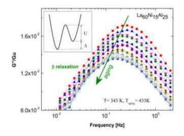
**Fig. 20.** Mechanical loss spectra of JG  $\beta$  relaxation in La<sub>60</sub>Ni<sub>15</sub>Al<sub>25</sub> amorphous alloy aged at 433 K with different aging time (Testing temperature is 343 K). Insert is schematic of asymmetric double well potential (ADWP) model [184]. Reprinted from [184], with the permission of AIP Publishing.
