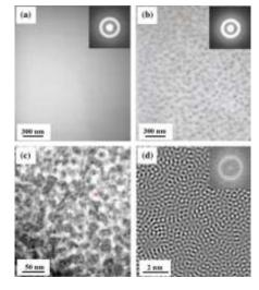
**Fig. 79.** Bright-field (BF)-transmission electron microscopy (TEM) images and selected-area diffraction patterns (SADPs) for the  $Cu_{47.2}Zr_{46.5}Al_{5.5}Nb_{0.8}$  amorphous alloy: (a) As-spun ribbon and (b) as-cast rod 2 mm in diameter. (c)Scanning transmission electron microscopy (STEM)-BF image showing the phase-separated
