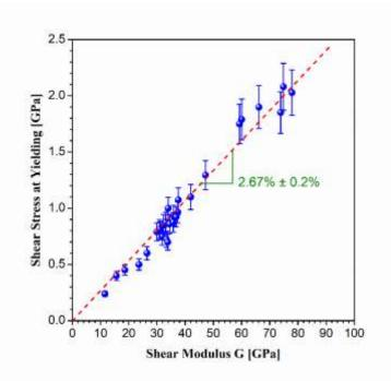
**Fig.69.** Experimental shear stress at yielding versus shear modulus G at room temperature in amorphous alloys [323]. Reprinted figures with permission from reference [323], copyright (2005) by the American Physical Society.
