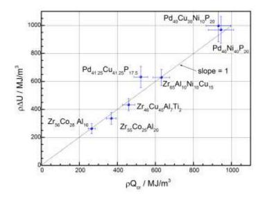
Fig. 61. Crystallization-induced change of the internal energy per unit volume  $\rho\Delta U$ as a function of the crystallization heat per unit volume  $\rho Q_{cr}$  for Pd- and Zr-based metallic glasses [371]. Reprinted from reference [371], copyright (2016), with permission from Elsevier.
