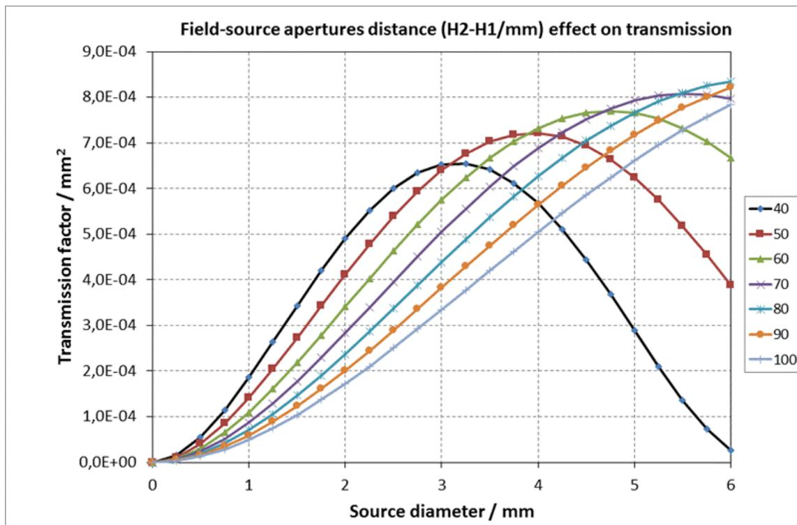
Figure 11 Influence of the distance  $L=H_2-H_1$  as mentioned at the right side in mm on the molecular transmission factor and for a fixed distance  $H_1$  between the effusion orifice and the field aperture. Refer to Figure 9 for the definition of the  $H_1$ ,  $H_2$  terms.
