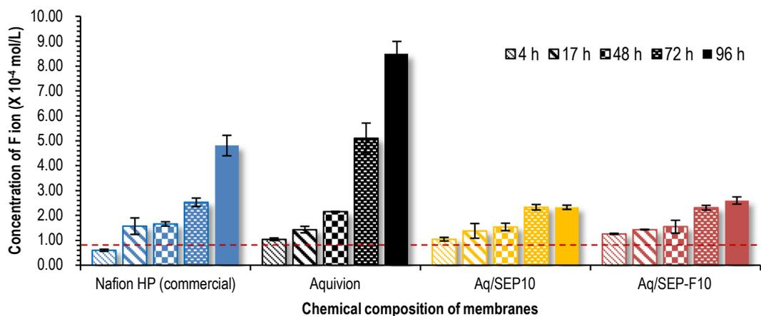
Fig. 8. Fluoride ( $F^-$ ) concentration analyzed after immersion in  $H_2O_2/H_2SO_4$  for Nafion HP, pristine Aquivion, Aq/SEP and Aq/SEP-F membranes. Red dotted line represents the fluorine concentration of 4.4 M  $H_2O_2/1.25$  mM  $H_2SO_4$  solution (blank test):  $0.82 \times 10^{-4} \pm 0.08 \times 10^{-4}$  mol/L.
