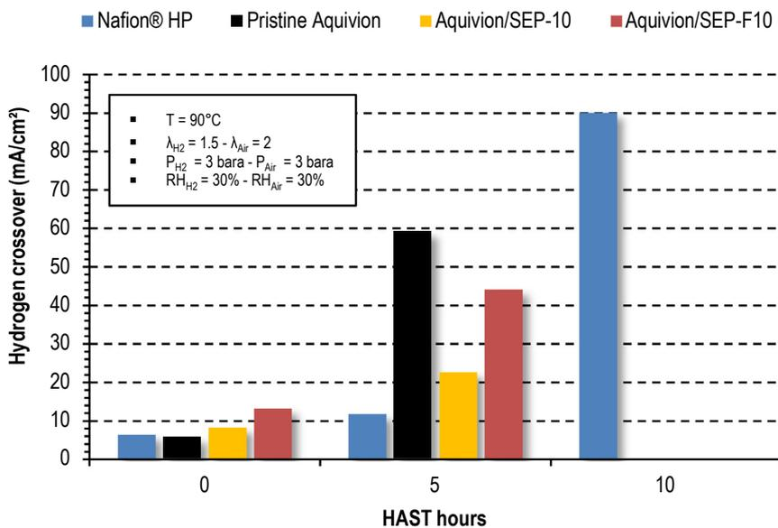
Fig. 11. Evolution of (a) the voltage at 0.6 A/cm<sup>2</sup> and (b) the hydrogen crossover for the different MEAs during the HAST.
