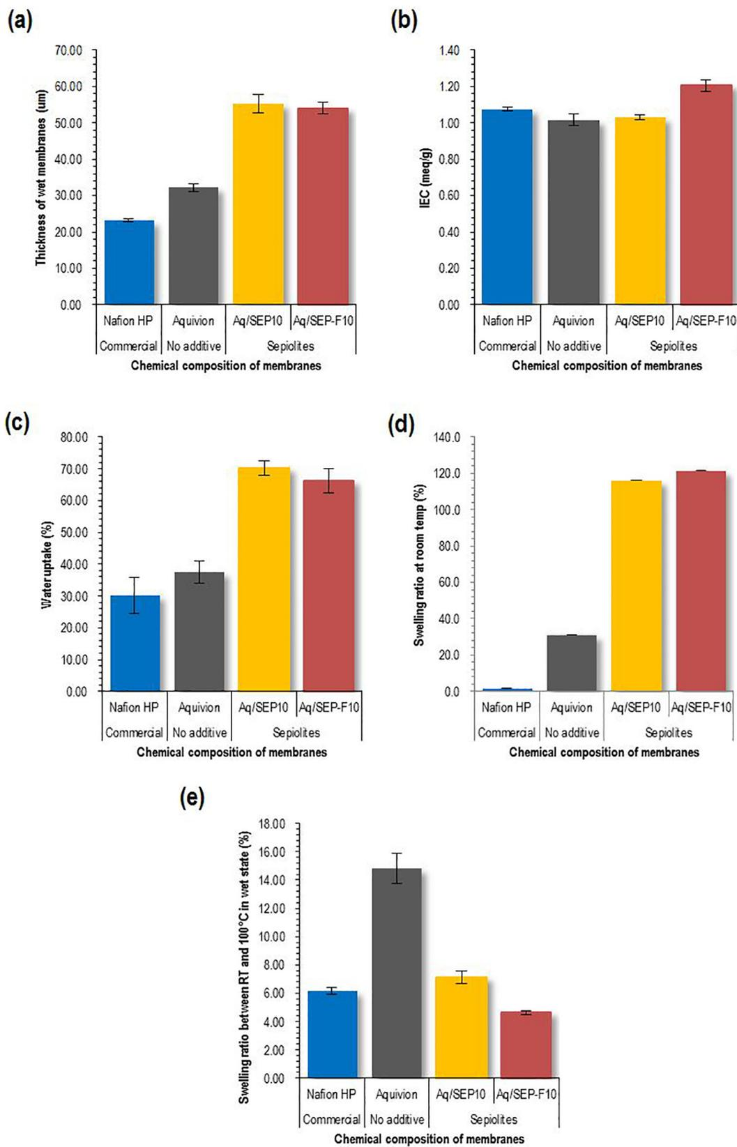
**Fig. 4.** Data on (a) thickness, (b) ion exchange capacity, (c) water uptake, (d) swelling between dry and wet states at room temperature and (e) swelling in wet state between room temperature and boiling water (100 °C): commercially available Nafion HP and pristine Aquivion and Aquivion composite membranes containing 10 wt% pristine and fluorinated sepiolites.
