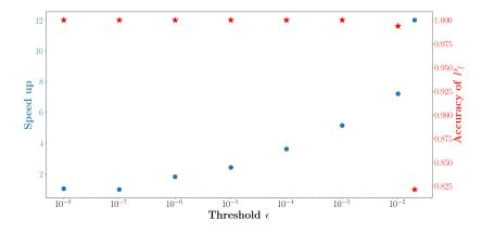
Figure 6: Accuracy (red stars) of  $P_f$  and speed up (blue dots) of the proposed method as a function of the threshold  $\epsilon$  on the non preconditioned residual for different constant DoEs and Monte Carlo generated by AK-MCS algorithm for the thermal problem.
