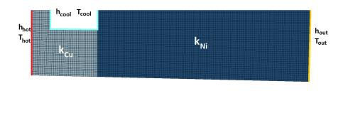
Figure 3: Finite element mesh of the combustion chamber wall and the boundary conditions of the thermal problem.
