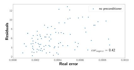
Figure 10: Correlation between the classical residual and the real error for the plate with a hole problem.
