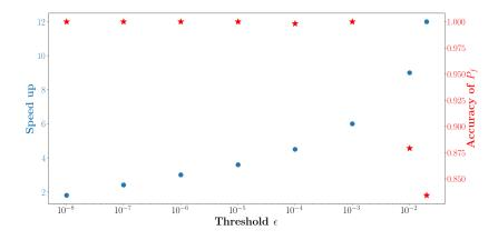
Figure 7: Accuracy (red stars) of  $P_f$  and speed up (blue dots) of the proposed method as a function of the threshold  $\epsilon$  on the preconditioned residuals for different constant DoEs and Monte Carlo generated by AK-MCS algorithm for the thermal problem.
