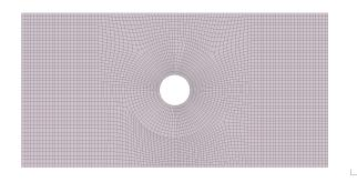
Figure 9: Finite element mesh of the laminated plate with a hole.
