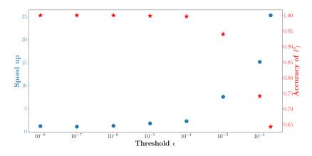
Figure 13: Accuracy (red stars) of the failure probability  $P_f$  and speed up (blue dots) as a function of the threshold  $\epsilon$  on the preconditioned residuals for different constant DoEs and Monte Carlo generated by AK-MCS algorithm for the laminated plate with a hole problem.
