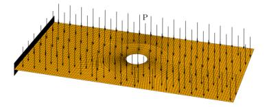
Figure 8: Boundary conditions and loading on the laminated plate.
