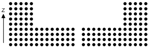
Fig. 3. Sketch of the multimode device: the large waveguide is obtained by removing seventeen rows of rods. The input single row and single-mode waveguide is used to inject the light.
