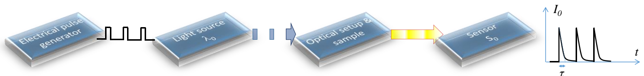
Fig. 2.50 Implementation for time resolved fluorescence spectroscopy
