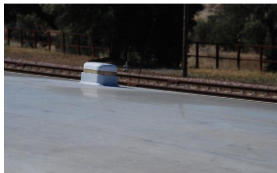
Figure 25 Final installation of GNSS antenna
