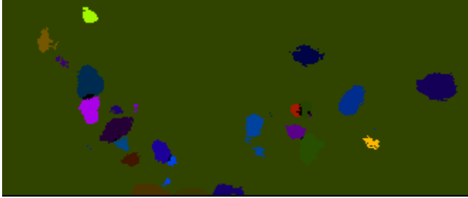
Fig. 6. A single slice through the grains shown in Fig. 4 showing relative spatial position of carbonado grains oriented in [110] direction ( \pm 15^\circ ).
