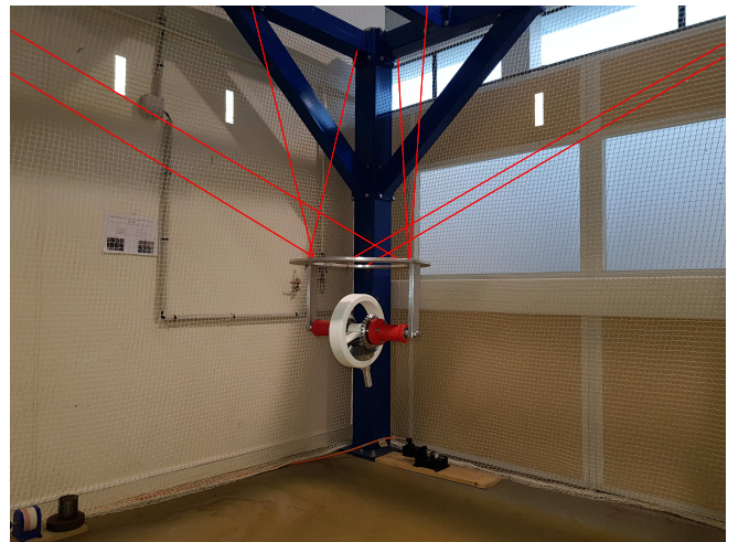
Figure 12: Prototype of the CDPR with an embedded tilt-roll wrist
