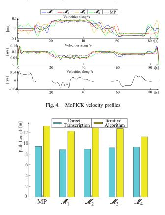
Fig. 5. Comparison of the path length between direct transcription and iterative algorithm.
