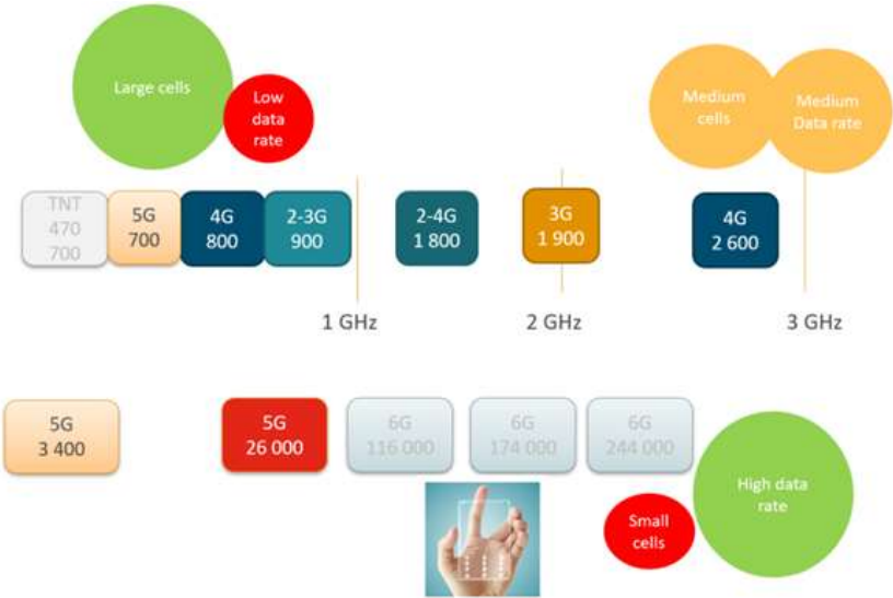
Fig. 10 - 2-5G mobile bandwidths, and prospective 6G bandwidths in 100 GHz range
