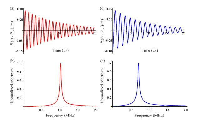
FIG. 9. Free oscillations of two equal bubbles. Left panel: bubbles in a cavity. Right panel: bubbles in an unbounded liquid.  $R_{10} = R_{20} = 5 \ \mu m$ ,  $z_1(0) = -50 \ \mu m$ ,  $z_2(0) = 50 \ \mu m$ ,  $R_{c0} = 100 \ \mu m$ ,  $R_s = 500 \ \mu m$ . The Minnaert frequency of the bubbles is 724 kHz. The free oscillations are excited by a small initial deviation from the equilibrium bubble radii.
