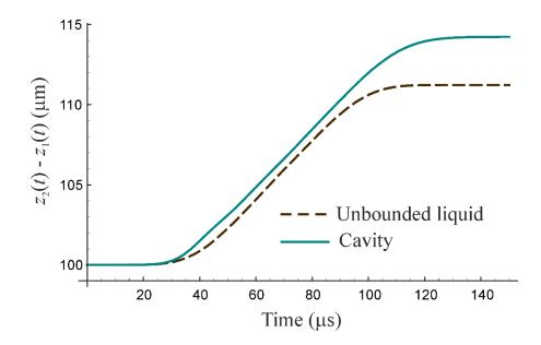
FIG. 6. Translational motion of two bubbles in a cavity and in an unbounded liquid. The parameters are as in Fig. 5, except that N = 50. The bubbles are moving away from each other.
