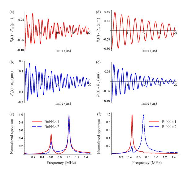
FIG. 10. Free oscillations of two unequal bubbles. Left panel: bubbles in a cavity. Right panel: bubbles in an unbounded liquid.  $R_{10} = 7.5 \ \mu m$ ,  $R_{20} = 5 \ \mu m$ ,  $z_1(0) = -50 \ \mu m$ ,  $z_2(0) = 50 \ \mu m$ ,  $R_{c0} = 100 \ \mu m$ ,  $R_s = 500 \ \mu m$ . The Minnaert frequencies of the bubbles are 468 kHz and 724 kHz.
