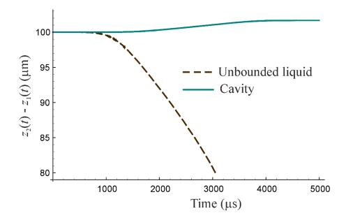
FIG. 8. Translational motion of two bubbles in a cavity and in an unbounded liquid. The parameters are as in Fig. 7, except that N = 1000.
