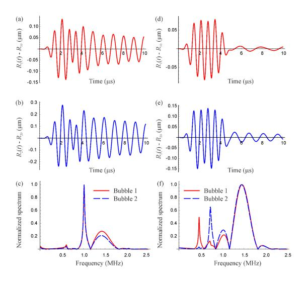
FIG. 3. Response of bubbles to the acoustic pulse shown in Fig. 2. Left panel: bubbles in a cavity. Right panel: bubbles in an unbounded liquid.  $R_{10} = 7.5 \ \mu m$ ,  $R_{20} = 5 \ \mu m$ ,  $z_1(0) = -50 \ \mu m$ ,  $z_2(0) = 50 \ \mu m$ ,  $R_{c0} = 100 \ \mu m$ ,  $R_s = 500 \ \mu m$ . The Minnaert frequencies of the bubbles are 468 kHz and 724 kHz. The bubbles are excited above their natural frequencies.
