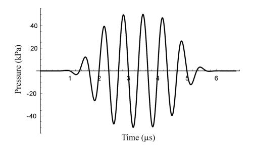
FIG. 2. Acoustic pulse used as excitation in Fig. 3. The mathematical definition is given by Eq. (32). The pulse parameters are f = 1.5 MHz,  $P_a = 50$  kPa, and N = 5.
