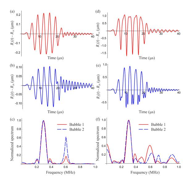
FIG. 7. Response of bubbles to an acoustic pulse with the parameters f = 0.3 MHz,  $P_a = 50$  kPa, N = 5. Left panel: bubbles in a cavity. Right panel: bubbles in an unbounded liquid.  $R_{10} = 7.5$  µm,  $R_{20} = 5$  µm,  $z_1(0) = -50$  µm,  $z_2(0) = 50$  µm,  $R_{c0} = 100$  µm,  $R_s = 500$  µm. The bubbles are excited below their natural frequencies.
