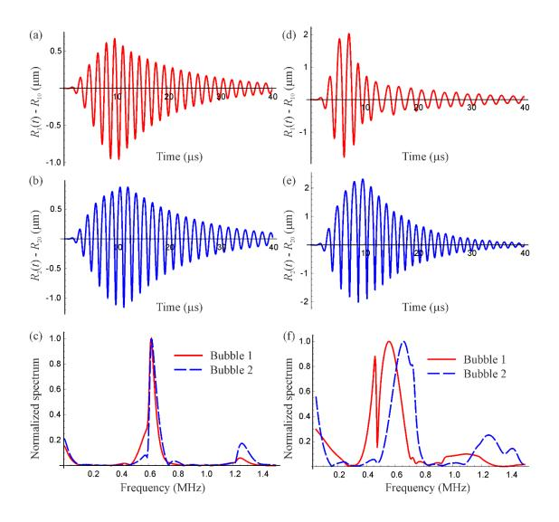
FIG. 5. Response of bubbles to an acoustic pulse with the parameters f = 0.6 MHz,  $P_a = 50$  kPa, N = 5. Left panel: bubbles in a cavity. Right panel: bubbles in an unbounded liquid.  $R_{10} = 7.5$  µm,  $R_{20} = 5$  µm,  $z_1(0) = -50$  µm,  $z_2(0) = 50$  µm,  $R_{c0} = 100$  µm,  $R_s = 500$  µm. The driving frequency lies between the natural frequencies of the bubbles.
