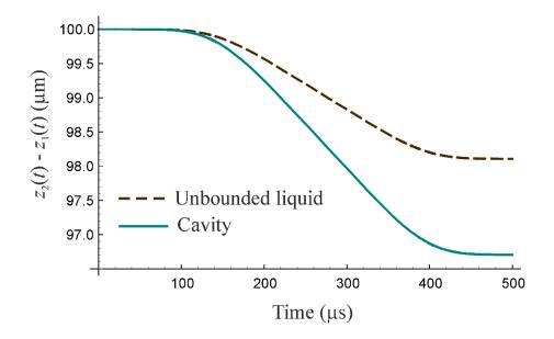
FIG. 4. Translational motion of two bubbles in a cavity and in an unbounded liquid. The parameters are as in Fig. 3, except that the number of cycles in the excitation pulse is N = 500. The bubbles are moving toward each other.
