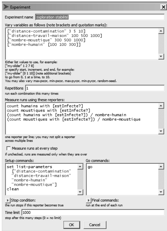
Figure 4.28. Defining an experiment plan allowing for a sensitivity analysis of the infection count
