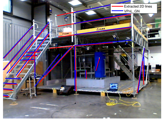
Fig. 7: Reprojection of 3D lines extracted from the Leica point cloud. The pose parameters are estimated with VPnL_GN only. 2D and 3D lines are paired manually.
