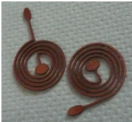
Figure 4. Copper spirals machined by EDM.
