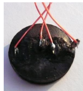
Figure 7. Coupler (ICT). Diameter 20 mm. Thickness 3 mm.
