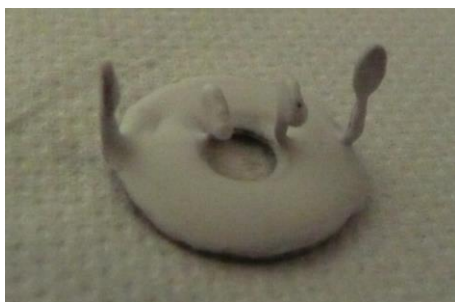
Figure 5. Spirals and washer covered with ceramic paint.
