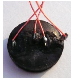
Figure 7. Coupler (ICT). Diameter 20 mm. Thickness 3 mm.
