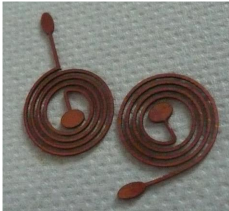
Figure 4. Copper spirals machined by EDM.
