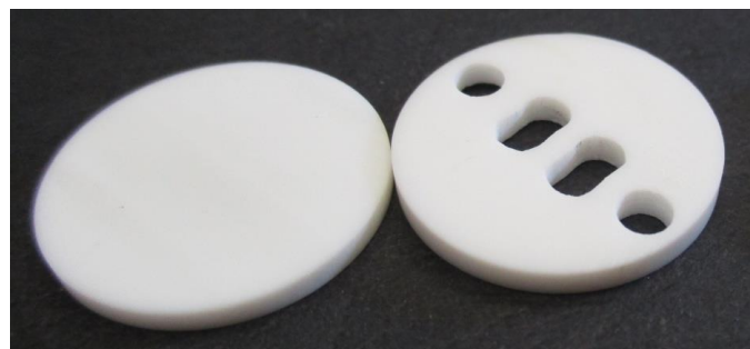
Figure 11. Alumina washer. Diameter 20 mm.
