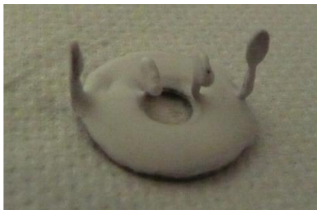
Figure 5. Spirals and washer covered with ceramic paint.
