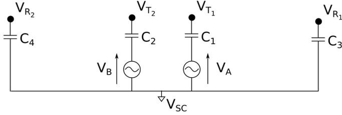
**Fig. 2.** Equivalent electrical arrangement of the emitters and receivers. This schematic does not correspond to the geometry considered in the electrostatic simulation (see Fig. 3).
