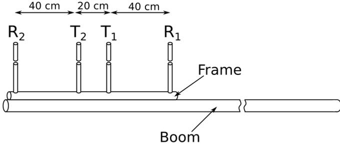
**Fig. 1.** Schematic of the mutual impedance probe mounted on its boom.
