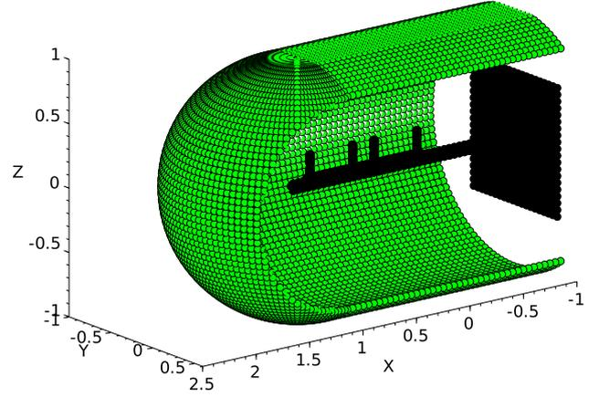
**Fig. 3.** Spatial configuration considered in the electrostatic simulations. The mutual impedance probe is located inside a cylindrical electron-free sheath ending by a hemisphere. The spacecraft body is modeled by the square plate. Plasma is only present at the external side of the sheath, which is presented in sectional view in order to show the probe.
