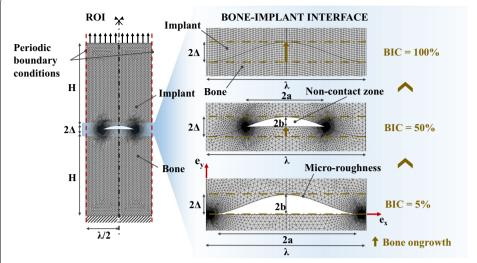
**Fig. 8** Mechanical and geometrical configurations of the FE model. Three phases of the bone ongrowth are sketched, corresponding to BIC = 5%, 50% and 100%
