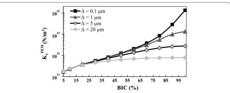
**Fig. 5** Variation of the numerical effective contact stiffness  $K_c^{\text{FEM}}$  as a function of the BIC for different values of the roughness amplitude Δ. The roughness wavelength  $\lambda$  and the bone Young's modulus  $E_b$  are equal to their reference values 80 μm and 2 GPa, respectively
