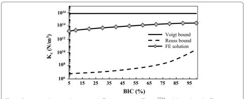
**Fig. 1** Comparison between the numerical effective contact stiffness  $K_c^{\text{FEM}}$  and the analytical stiffness obtained from the Voigt–Reuss bounds [see Eqs. (7)–(10)] as a function of the BIC. The roughness wavelength  $\lambda$ , amplitude  $\Delta$  and the bone Young's modulus  $E_b$  are equal to their reference values 80 μm, 5 μm and 2 GPa, respectively
