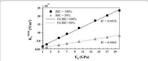
**Fig. 7** Variation of the numerical effective contact stiffness  $K_c^{\mathsf{FEM}}$  as a function of the bone Young's modulus  $E_b$  for different values of the BIC. The roughness amplitude  $\Delta$  and the wavelength  $\lambda$  are equal to their reference values 5  $\mu$ m and 80 GPa, respectively
