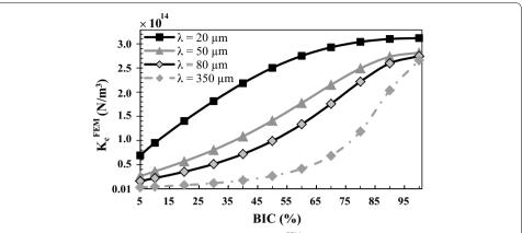
**Fig. 6** Variation of the numerical effective contact stiffness  $K_c^{\text{FEM}}$  as a function of the BIC for different values of  $\lambda$ . The roughness amplitude  $\Delta$  and the bone Young's modulus  $E_b$  are equal to their reference values 5 μm and 2 GPa, respectively
