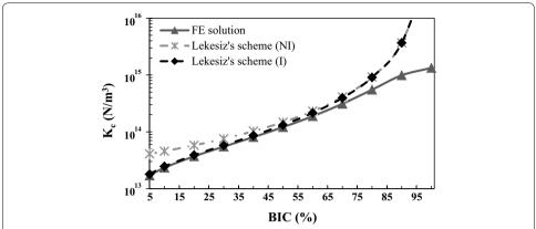
**Fig. 4** Variation of the effective contact stiffness  $K_C$  obtained with the finite element model, the Lekesiz's model with crack interaction (I) and the Lekesiz's model without crack interaction (NI) as a function of the BIC. The roughness amplitude  $\Delta$  is equal to 1  $\mu$ m; the roughness wavelength  $\lambda$  and the bone Young's modulus  $E_b$  are equal to their reference values 80  $\mu$ m and 2 GPa, respectively
