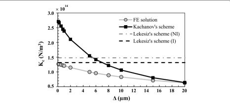
**Fig. 2** Variation of the effective contact stiffness  $K_C$  obtained with the finite element model, the Kachanov's model, the Lekesiz's model with crack interaction (I) and the Lekesiz's model without crack interaction (NI) as a function of the roughness amplitude Δ. The roughness wavelength  $\lambda$ , the BIC and the bone Young's modulus  $E_b$  are equal to their reference values 80 μm, 50% and 2 GPa, respectively
