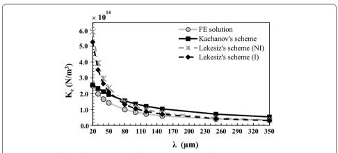
**Fig. 3** Variation of the effective contact stiffness  $K_C$  obtained with the finite element model, the Kachanov's model, the Lekesiz's model with crack interaction (I) and the Lekesiz's model without crack interaction (NI) as a function of the roughness wavelength  $\lambda$ . The roughness amplitude  $\Delta$ , the BIC and the bone Young's modulus  $E_b$  are equal to their reference values 5 μm, 50% and 2 GPa, respectively
