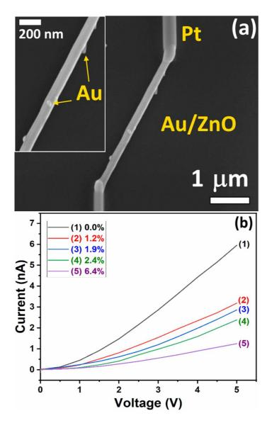
**Figure 1**. (a) SEM image of a nanophotodetector based on an individual Au/ZnO NW with a radius of 75 nm. The inset presents a zoomed region with Au NPs attached on the surface of the NW. (b) Current – voltage (*I–V*) characteristics of individual Au/ZnO NWs with different Au NPs coverage.
