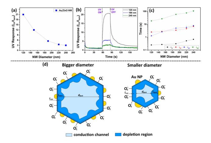
**Figure 3**. (a) UV response of individual Au/ZnO NWs versus diameter of the nanowire integrated in nanosensor. (b) Dynamic UV response of individual Au/ZnO NWs with different diameters. (c) The calculated time constants for rising and decaying photocurrent of individual Au/ZnO NWs with different diameters. (d) The UV sensing mechanism based on different diameter (bigger and smaller one) of an Au/ZnO NW used in nanosensors in cross-sectional view.
