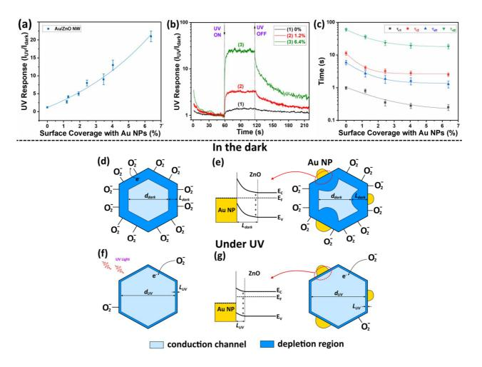
**Figure 2**. (a) Measured UV response of individual Au/ZnO NWs (with D = 120 nm) versus Au NPs coverage on the surface of NW. (b) Dynamic UV response of individual Au/ZnO NWs with different Au NPs coverage on the surface. (c) The calculated time constants of rising and decaying photocurrent for individual Au/ZnO NWs. The UV sensing mechanism of individual ZnO NW and Au/ZnO NW: ZnO NW in the dark (d) and under UV illumination (f); Au/ZnO NW in the dark (e) and under UV illumination (g).
