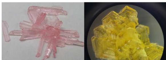
Figure 3. Crystal of two mixed metal chlorides: a) \text{KMnCl}_3 and b) \text{K}_3\text{NaMnCl}_6 from \text{Eco-Mn}_{\text{LA}} identified by XRD analyses.
