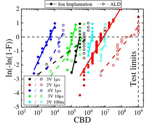
Fig. 13: CBD distribution of ALD 30:1 2,38% and II  $3,0e14$  at/cm $^2$  1,39% with 5 different pulse conditions and  $tr/ta = 100ns$ .
