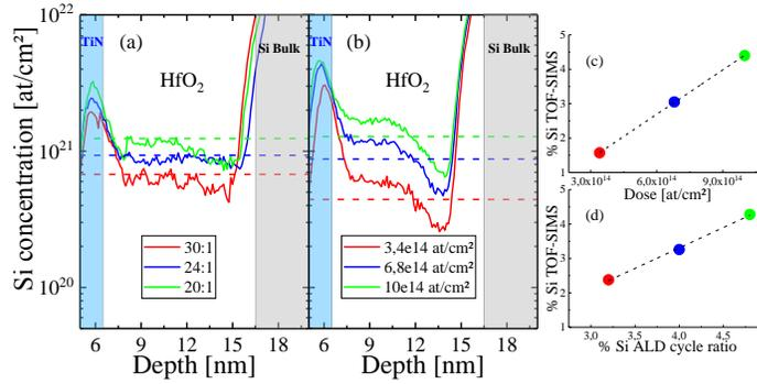
Fig. 2: Si implanted profiles for (a) the ALD case and (b) the II case. The dashed lines represent the averaged concentration. %Si extracted by this methodology is plotted in (c) for the II case and (d) for the ALD case, with corresponding linear regression (dashed lines).
