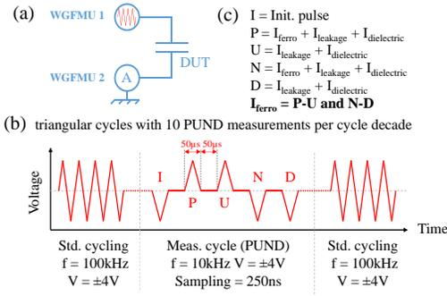
Fig. 3: (a) Schematic representation of measurement setup, based on 2 Keysight B1530 Waveform Generator/Fast Measurement Units (WGFMU) (b) Applied test sequence: triangular waking-up cycles ( $\pm 4\text{V}/100\text{kHz}$ ) with PUND ( $\pm 4\text{V}/10\text{kHz}$ ) ferroelectric measurements performed 10 times per cycle decade. (c) PUND measurement description for correcting leakage and dielectric displacement current contributions.
