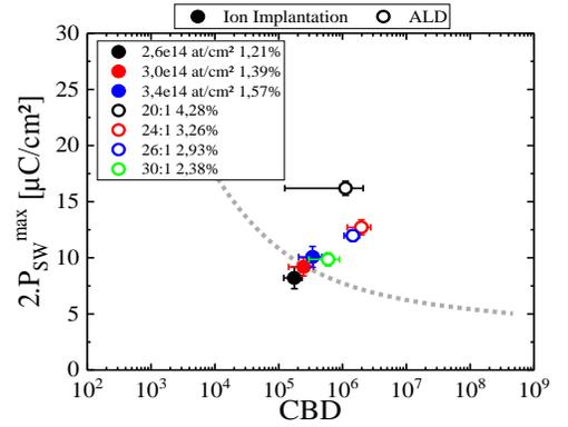
Fig. 16:  $2.P_{sw}^{max}$  achieved during optimized square cycling, 3V/1µs and  $tr/ta = 100ns$ , as a function of the corresponding CBD, for all doping conditions. The dashed line corresponds to the previous trend of Fig. 14.
