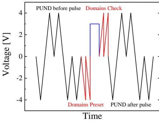
Fig. 9: Sequence used, after  $10^4$  wake-up signal 4V/100kHz, to evaluate the switching efficiency of square pulses. The PUND 4V/10kHz are used as polarization references. The domains preset signal ensure the initialization of the opposite state, while the domains check signal measure the polarization which has not been switched by the pulse. Both checks are double ramp to perform a PUND-like extraction, cf. Fig. 3 (c).
