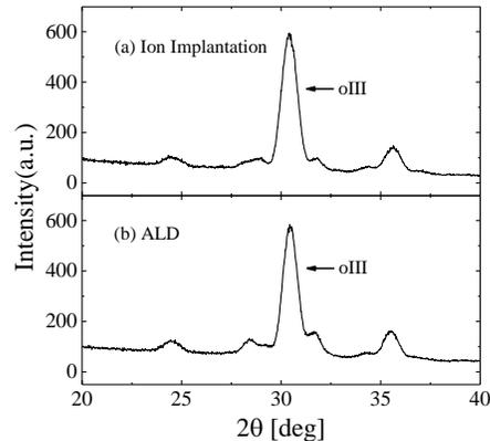
Fig. 6: GIXRD measurement of (a) Ion Implantation  $3.4 \times 10^{14}$  at/cm<sup>2</sup> and (b) ALD 30:1. The ferroelectric orthorhombic oIII-phase peaks confirm the electrical measurement for both doping techniques.
