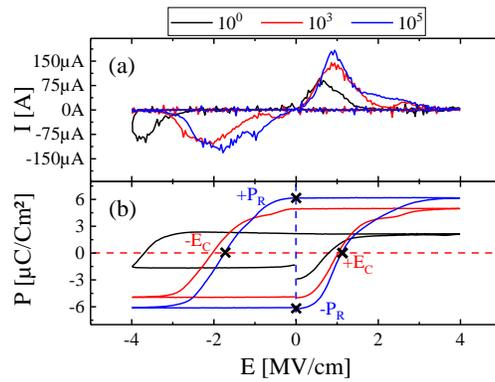
Fig. 4: For the ALD case 30:1 2,38% Si, (a) I-E at (black)  $10^0$ , (red)  $10^3$  and (blue)  $10^5$  cycles obtained by PUND technique where typical ferroelectric peaks are visible and (b) corresponding P-E with the ferroelectric metrics, i.e.  $P_R^{+/-}$  and  $E_C^{+/-}$ , highlighted by the marks.
