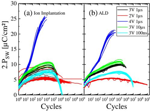
Fig. 11:  $2.P_{sw}$  along cycling of (a) II  $3,0e14$  at/cm $^2$  1,39% and (b) ALD 30:1 2,38% with 5 different pulse conditions and  $tr/ta = 100ns$ .
