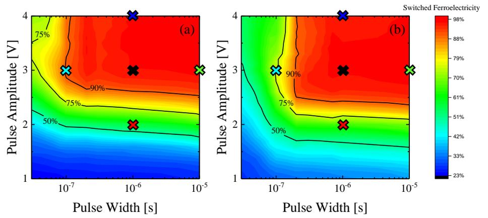
Fig. 10: Switching efficiency maps of (a) ALD 30:1 2,38% and (b) II  $3,0e14$  at/cm $^2$  1,39% with  $tr/ta = 100ns$ . These devices have the same behavior along wake-up cycling according to Fig.5 (a). The marks indicate the chosen parameters for the following study.
