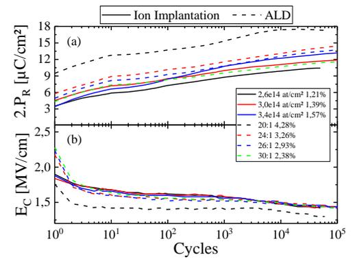
Fig. 5: (a) median  $2.P_R$  and (b) median  $E_C$  along triangular wake-up cycling  $4\text{V}/100\text{kHz}$  for all doping conditions extracted 10 times by decade by a PUND read signal at  $4\text{V}/10\text{kHz}$ . Straight lines correspond to II while dashed lines are for ALD.
