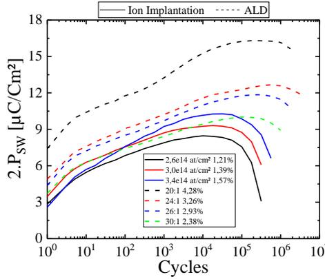
Fig. 15: Median  $2.P_{sw}$  along optimized square cycling 3V/1µs and  $tr/ta = 100ns$  for all doping conditions extracted 5 times by decade.
