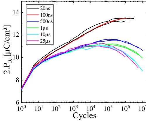
Fig. 12: Impact of the  $tr/ta$  along cycling for 24:1 3,26% case. The pulse parameters are 3V/1µs for every measure.
