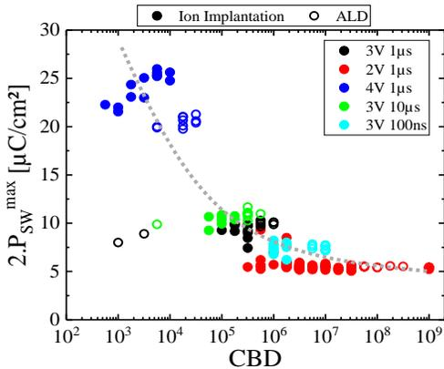
Fig. 14:  $2.P_{sw}^{max}$  achieved during square cycling with various conditions and  $tr/ta = 100ns$  as a function of the corresponding die's CBD. Tested devices are ALD 30:1 2,38% and II  $3,0e14$  at/cm $^2$  1,39%. The trend is highlighted by the dashed line.
