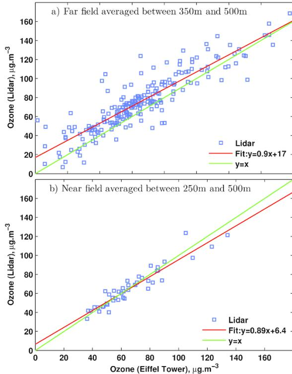
**Fig. 1:** Scatter plot of ozone concentrations measured by the Lidar and the Eiffel Tower measurements between 2011 and 2014. Top panel shows the Lidar far field (large telescope) averaged between 350m and 500m and the bottom panel shows the Lidar near field (small telescope) averaged between 250m and 500m.
