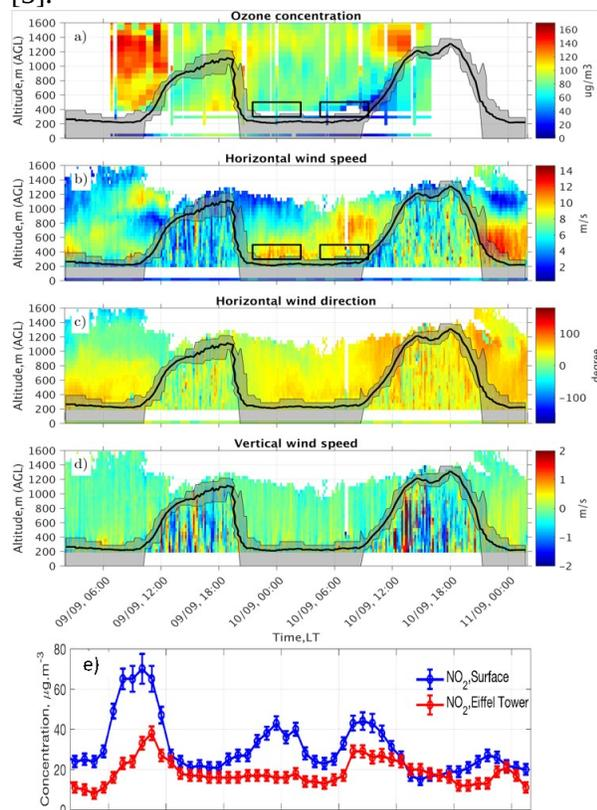
**Fig. 3:** Time evolution on 9 and 10 September of lidar O<sub>3</sub> concentrations (a), of surface O<sub>3</sub> (a) and NO<sub>x</sub> (e) measured at the Eiffel Tower (275m AGL) and the Paris13 station (5m AGL), of the horizontal lidar wind speed (b) and direction (c), of vertical wind speed (d). Surface wind speed and direction measured at Montsouris are also shown in (b) and (c). The PBL height is shown in black with its uncertainty in grey.
