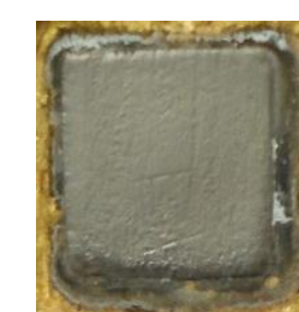
Fig. 3 – electrodeposited Ni/Ga alloy on gold substrate
