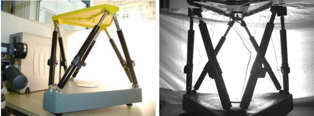
Fig. 13. A photograph of a Gough-Stewart platform (left) and a current configuration seen from the camera (the desired configuration is in the background).
