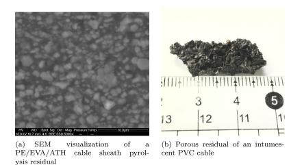
Figure 1: Illustration of the morphology of pyrolysis residuals for two different materials
