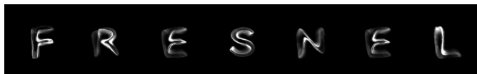
Fig. 5. Letters of the Latin alphabet can be obtained with electrically driven plasmonic nanoscatterers. To display the word FRESNEL, each letter is first obtained individually before assembling the 7 images to form the word.
