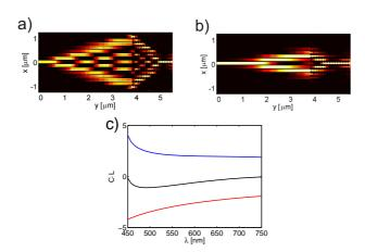
Fig. 4. (Color online) Time average power flow in y direction (normalized to the maximum) in the diffraction managed device at different wavelengths: a) 450nm, b) 750nm. c) Diffraction coefficient times propagation length  $(C \cdot L)$  for array A1 (red), array A2 (blue) and for the entire device  $(C_1 \cdot L_1 + C_2 \cdot L_2)$  (black).
