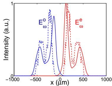
Fig. 4. Solitonic decay,  $I = 2.5 \text{ GW/cm}^2$ . Experimental (dashed lines) and numerical (solid lines) spatial output profiles at the exit face of the KTP crystal along  $x$ , intersection between the exit face of the crystal and the ordinary plane.  $E_{\omega}^e$  (red lines), and  $E_{\omega}^o$  (blue lines).
