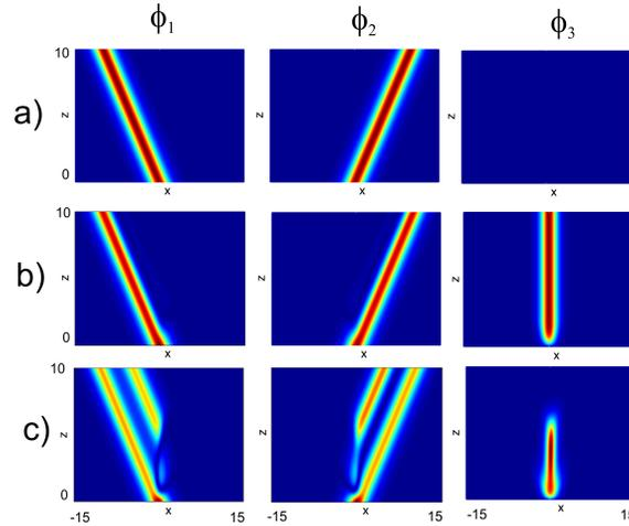
Fig. 1. Numerical  $x-z$  TWRI dynamics of waves at frequency  $\omega_1$  and  $\omega_2$  which mix to generate a field at the sum frequency  $\omega_3$ . (a) Linear, (b) frequency conversion, and (c) solitonic regime.
